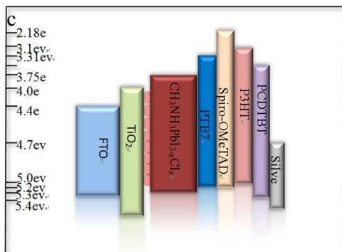
Figure 1 (a) device structure diagram of the FTO / c-TiO 2 / m-TiO 2 / CH 3 NH 3 PbI 3-x Cl x / PTB7 / Spiro-OMeTAD / P3HT / PCDTBT / Silver; (b) the cross-section SEM image of the whole device; (c) corresponding energy level alignment of the device.
