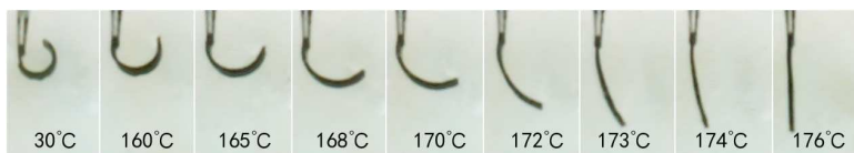
Fig 12 shape recovery process pictures for (2)/DDM from 30°C to 176°C in silicone oil at a heating rate of 10°C/min.
