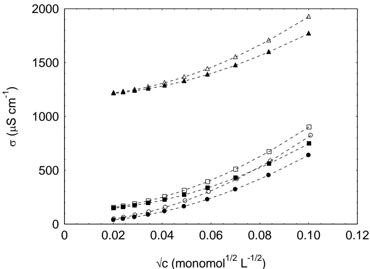
**Fig. 2** Experimental specific conductivities ( $\kappa$ ) of NaPSS in the presence of varying concentrations of NaCl [0.0001 (circles), 0.0010 (squares), and 0.0100 (triangles) mol L<sup>-1</sup>] in water as a function of the square root of the polyelectrolyte concentration at 298.15 K. The open symbols refer to the NaPSS sample with a molecular weight of 70000 whereas the closed symbols to the NaPSS sample with a molecular weight of 1000000.
