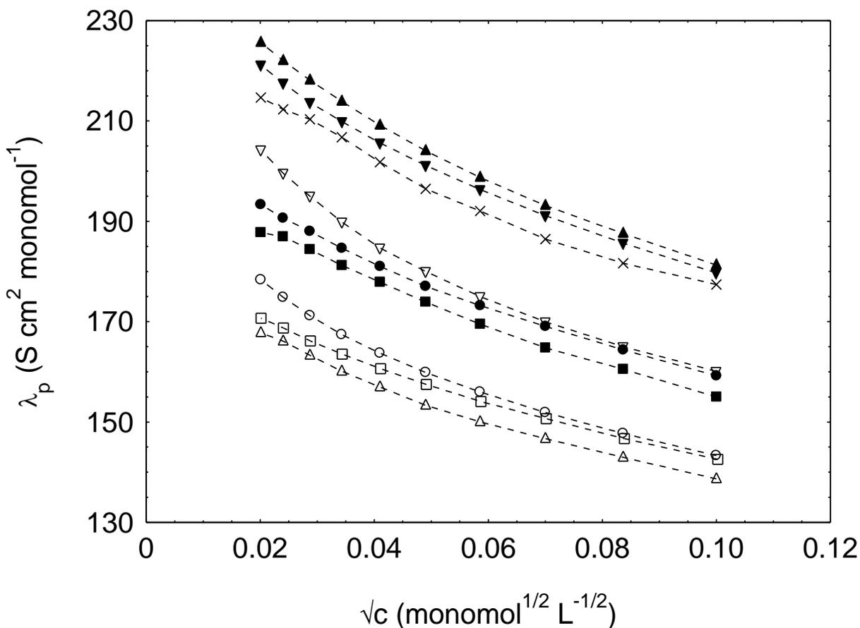
**Fig. 4(b)** Polyion equivalent conductivity in aqueous solution of NaPSS (molecular weight = 1000000) in presence of NaCl at different temperatures. For the significance of symbols, please refer to Fig. 3(a).
