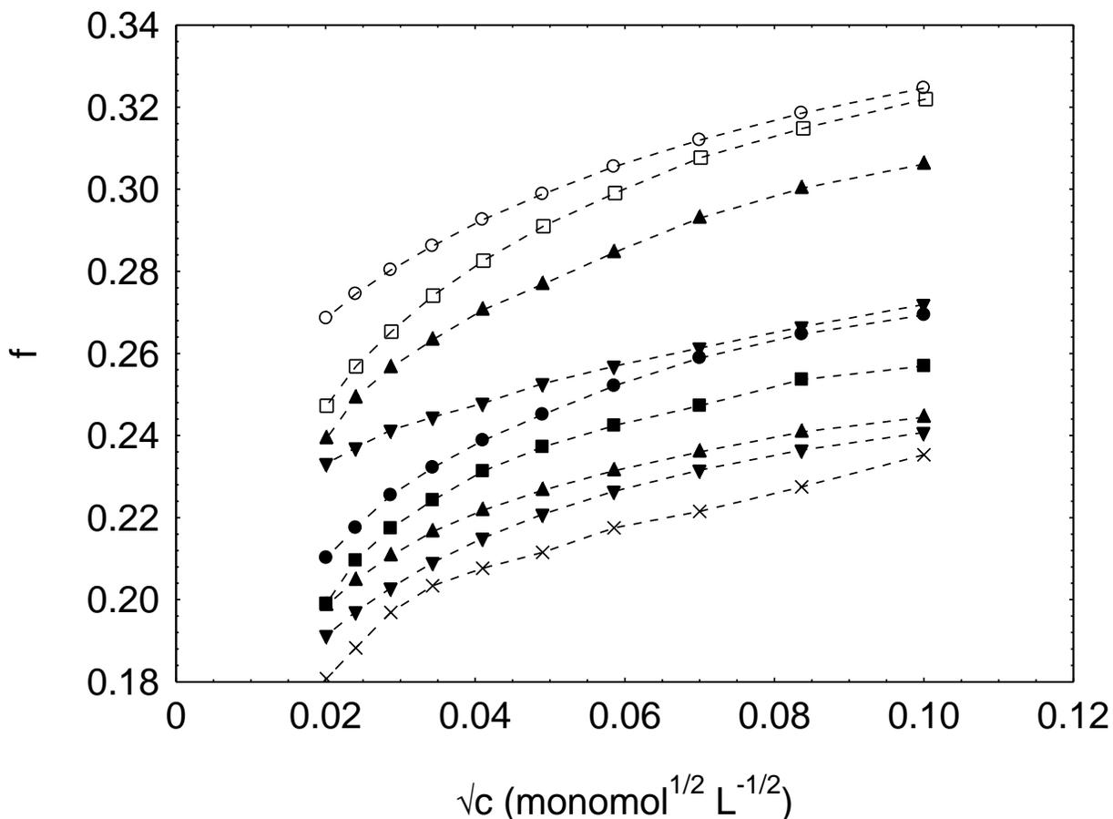
**Fig. 3(b)** Fraction of free counterions in aqueous solution of NaPSS (molecular weight = 1000000) in presence of NaCl at different temperatures. For the significance of symbols, please refer to Fig. 3(a).
