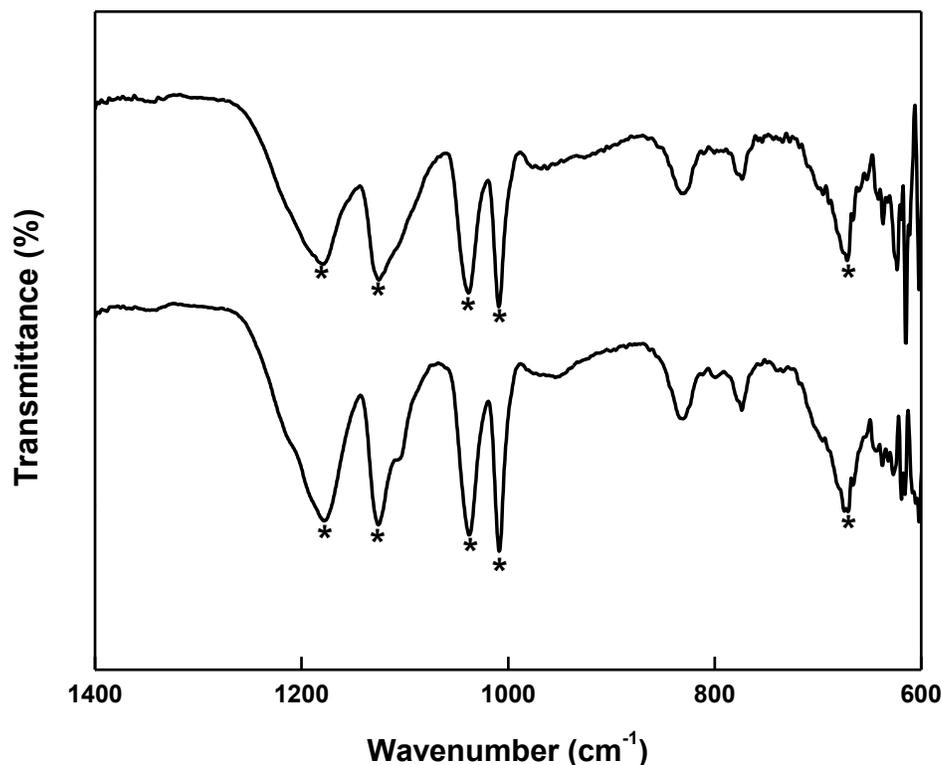
**Fig. 1** FT-IR spectra NaPSS samples: Molecular weight 70000 (top spectrum) and 1000000 (bottom spectrum).
