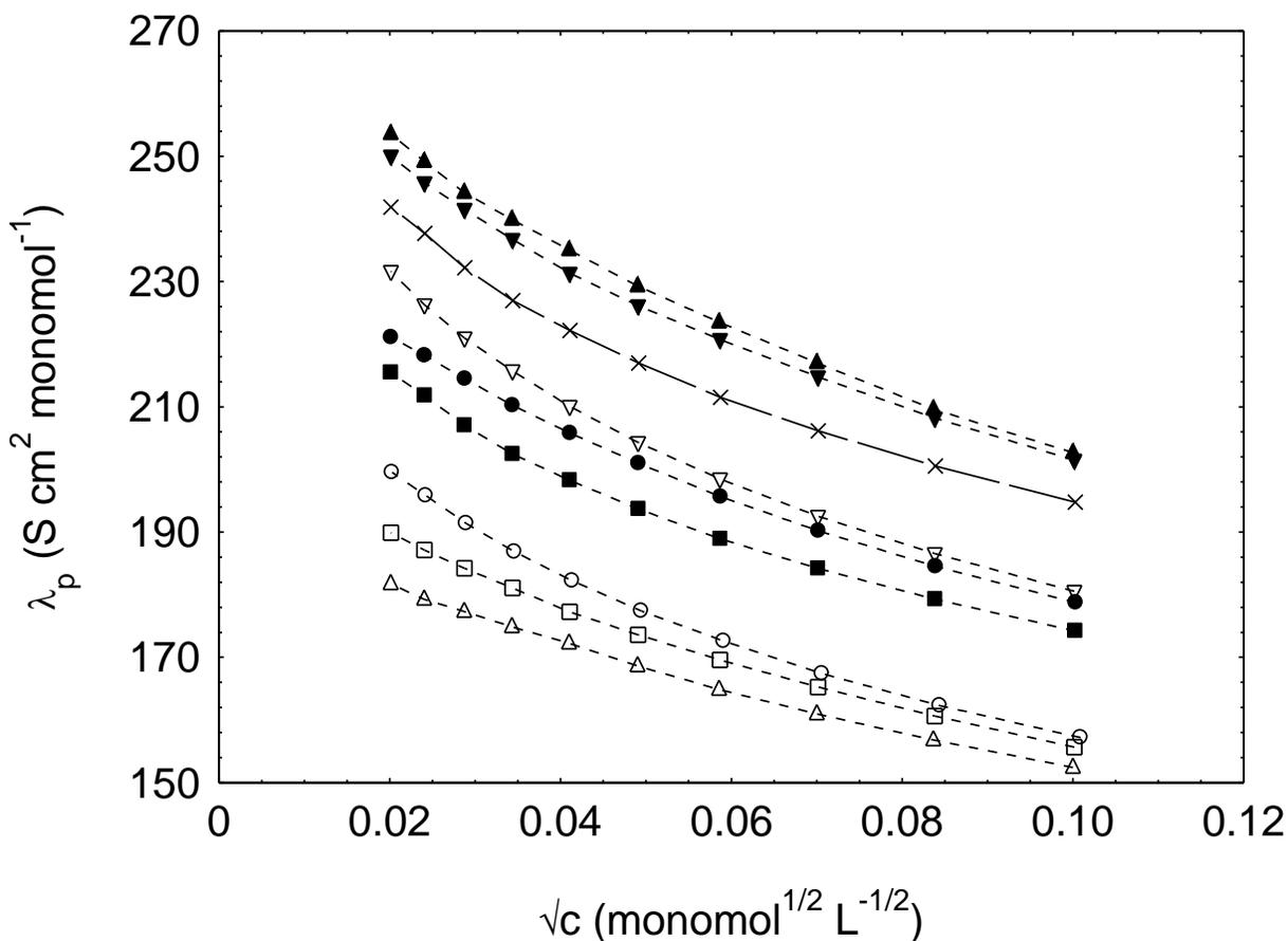
**Fig. 4(a)** Polyion equivalent conductivity in aqueous solution of NaPSS (molecular weight = 70000) in presence of NaCl at different temperatures. For the significance of symbols, please refer to Fig. 3(a).
