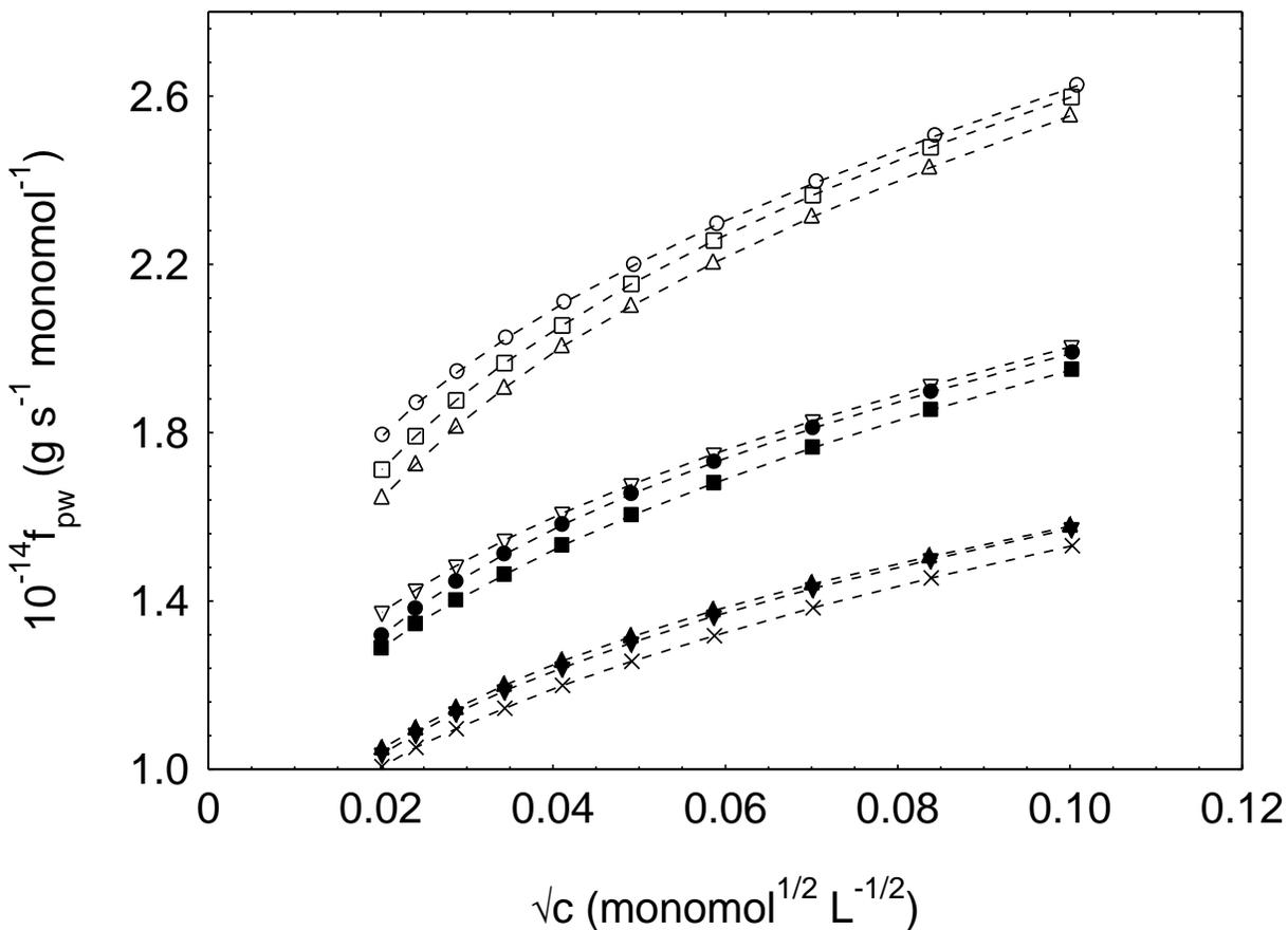
**Fig. 5 (a)** Coefficient of friction between polystyrenesulfonate ion and the solvent in aqueous solution of NaPSS (molecular weight = 70000) in presence of NaCl at different temperatures. For the significance of symbols, please refer to Fig. 3 (a).
