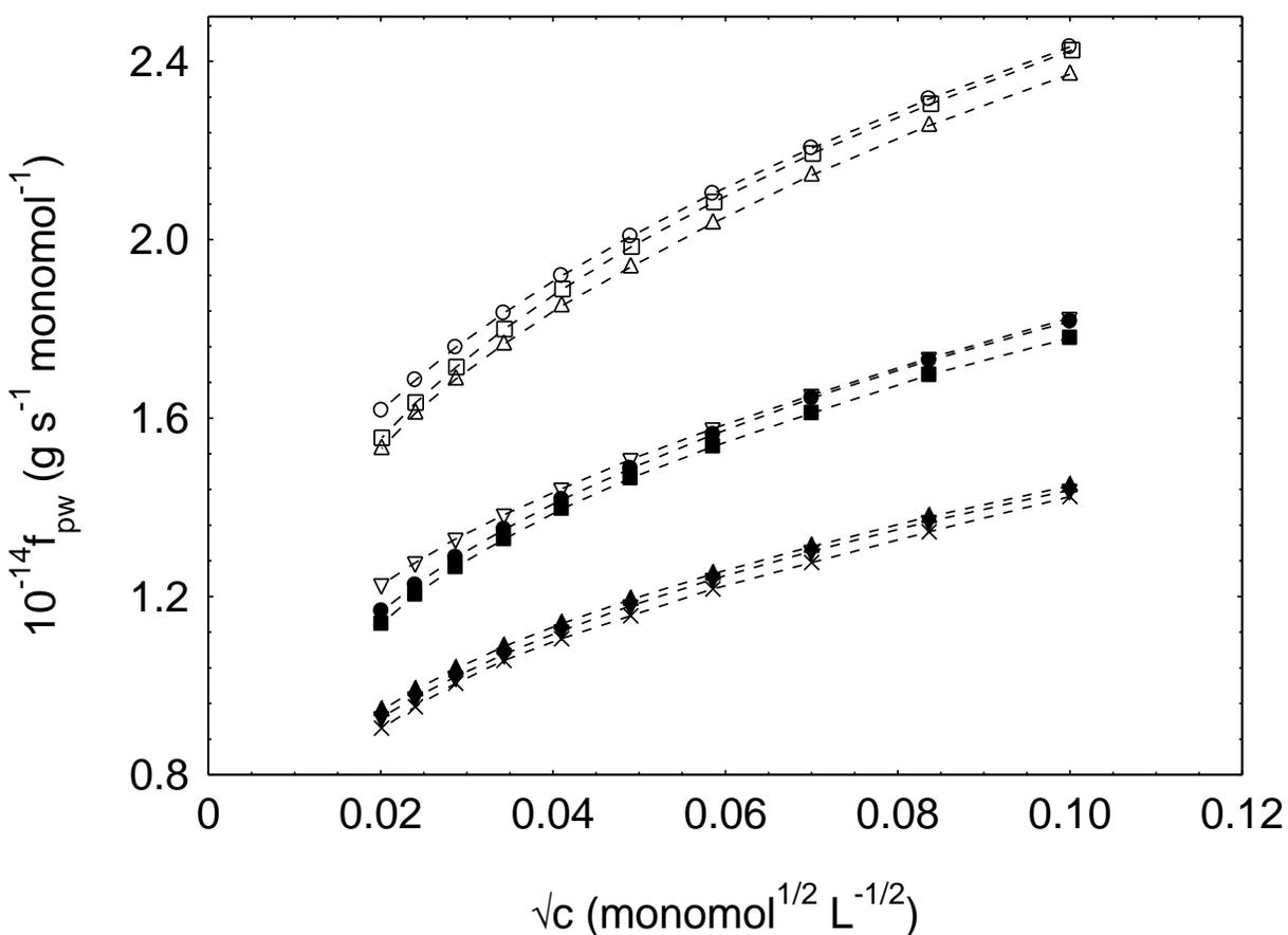
**Fig. 5 (b)** Coefficient of friction between polystyrenesulfonate ion and the solvent in aqueous solution of NaPSS (molecular weight = 1000000) in presence of NaCl at different temperatures. For the significance of symbols, please refer to Fig. 3 (a).
