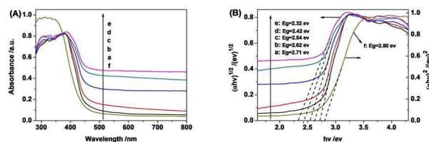
Fig. 3 UV-vis DRS (A) and plots of  $(\alpha hv)^{1/2}$  vs. photon energy (B) of g-C<sub>3</sub>N<sub>4</sub> (a), P-C<sub>3</sub>N<sub>4</sub> (b), CeO<sub>2</sub>(7.4%)/P-C<sub>3</sub>N<sub>4</sub> (c), CeO<sub>2</sub>(13.8%)/P-C<sub>3</sub>N<sub>4</sub> (d), CeO<sub>2</sub>(19.4%)/P-C<sub>3</sub>N<sub>4</sub> (e) and plot of  $(\alpha hv)^2$  vs. photon energy (B) of CeO<sub>2</sub>(f).
