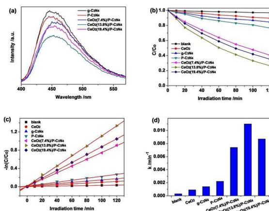
Fig. 4 PL spectra (a) of as-prepared photocatalysts, photocatalytic activities (b) of as-prepared photocatalysts for the photodegradation of MO in aqueous solution under visible light irradiation ( $\lambda \geq 420$  nm), first-order kinetics plot (c) and the kinetic constants (d) for the photodegradation of MO in aqueous solution over as-prepared photocatalysts.
