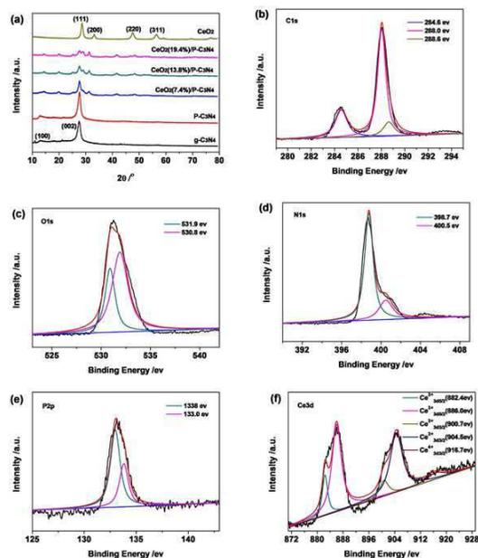
Fig. 2 XRD patterns (a) of the as-prepared photocatalysts, C1s (b), O1s (c), N1s (d), P2p (e) and Ce3d (f) XPS spectrum of the CeO<sub>2</sub>(13.8%)/P-C<sub>3</sub>N<sub>4</sub> photocatalyst.
