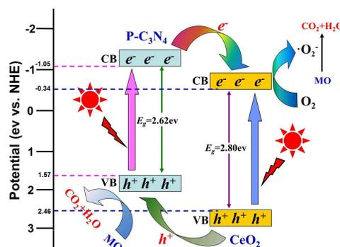
Fig. 6 Schematic illustration of the charge transfer pathway of the CeO<sub>2</sub>/P-C<sub>3</sub>N<sub>4</sub> composite catalyst under visible light irradiation.
