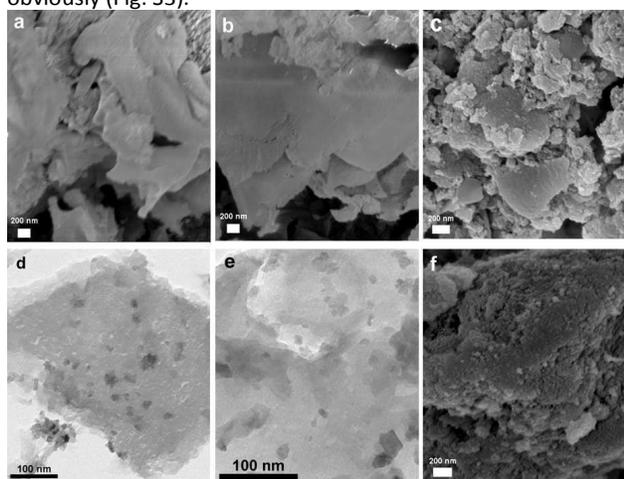
Fig. 1 SEM (a, b, c and f) and TEM (d and e) images of g-C<sub>3</sub>N<sub>4</sub> (a), P-C<sub>3</sub>N<sub>4</sub> (b), CeO<sub>2</sub>(13.8%)/P-C<sub>3</sub>N<sub>4</sub> (c and d), CeO<sub>2</sub>(13.8%)/P-C<sub>3</sub>N<sub>4</sub> used for 4th cycle (e) and CeO<sub>2</sub> (f).
