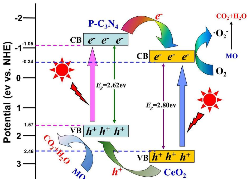
CeO<sub>2</sub>/P-C<sub>3</sub>N<sub>4</sub> composite catalysts exhibited excellent photocatalytic activity and stability for the photocatalytic degradation of methyl orange under visible light irradiation ( $\lambda > 420\text{ nm}$ ), arising from the synergistic effect between P-C<sub>3</sub>N<sub>4</sub> and CeO<sub>2</sub>, which effectively improved photogenerated electron-hole pairs separation efficiency.
