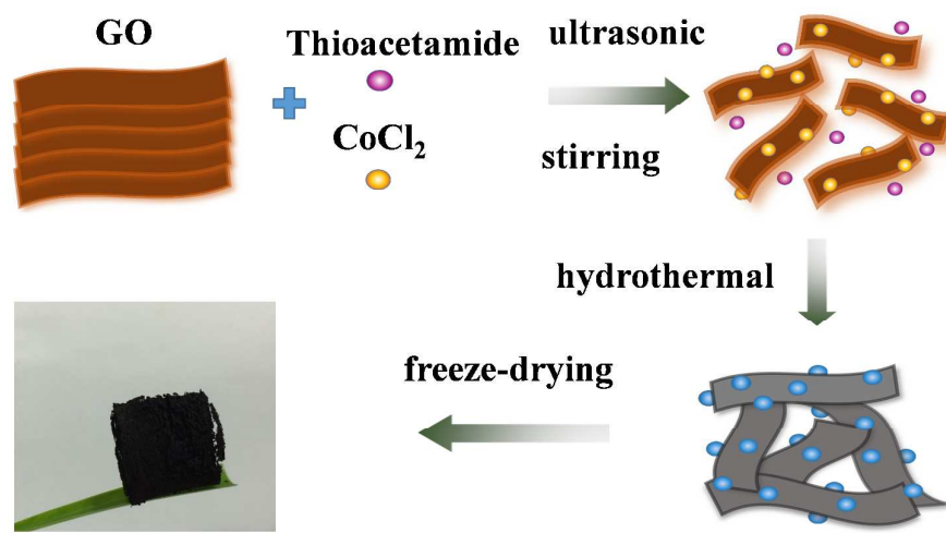
Fig.1 Schematic illustration of the synthesis of 3DCG.
