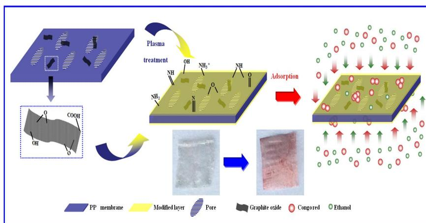
Through a plasma treatment, a PP-based composite membrane with a high hydrophilicity and an excellent adsorption ability was developed.
