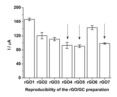
Fig. 11 ASWV peak currents of Pu(IV)/Pu(III) redox couple recorded on seven rGO/GCs in the final test solution (i.e.; Sample + 3.047 mg g<sup>-1</sup> of standard Pu). The error bars represent the standard deviation for ten repetitive measurements. The arrows show the rGO/GCs selected for the ANOVA test.
