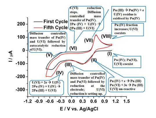
Schematic representation of the interference of Pu(IV) in the voltammetric determination of U in a mixed U-Pu solution in 1 M  $H_{So.}$
