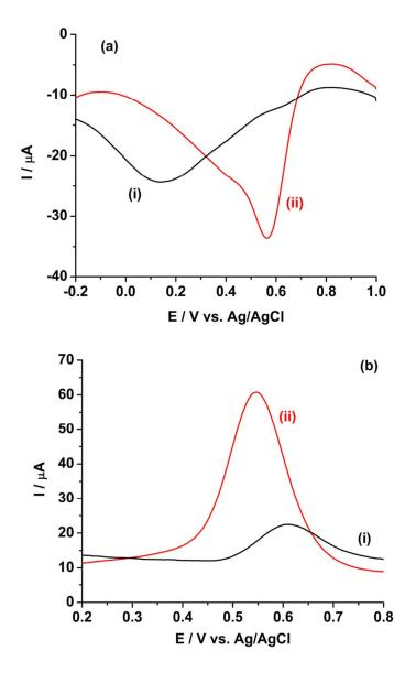
**Fig. 4** Square wave voltammograms of 10 mM Pu(IV) in 1 M  $H_2SO_4$  solution on (i) GC and (ii) rGO/GC electrodes in the (a) cathodic and (b) anodic scan directions. Square wave amplitude = 25 mV; Square wave frequency = 20 Hz; Step potential increment = 1 mV; Hold time at initial potential = 10 s.
