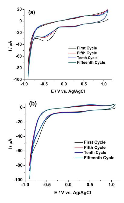
**Fig. 8** Cyclic voltammograms of 5 mM U(VI) in 1 M  $H_2SO_4$  on (a) rGO/GC and (b) GC electrodes at a scan rate of 50 mV s<sup>-1</sup> for (i) first, (ii) fifth, (iii) tenth and (iv) fifteenth cycle.
