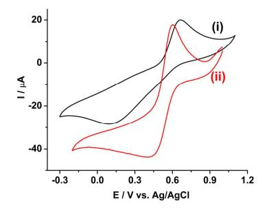
Fig. 1 Cyclic voltammograms of 10 mM Pu(IV) in 1 M  $H_2SO_4$  solution on (i) GC and (ii) rGO/GC electrodes at a scan rate of 10 mV s<sup>-1</sup>.
