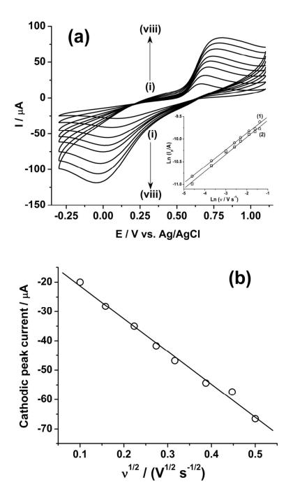
**Fig. 2 (a)** Cyclic voltammograms of 10 mM Pu(IV) in 1 M H<sub>2</sub>SO<sub>4</sub> solution on GC electrodes at a scan rate ( $\upsilon$ ) of (i) 10, (ii) 25, (iii) 50, (iv) 75, (v) 100, (vi) 150, (vii) 200 and (viii) 250 mV s<sup>-1</sup>. The inset shows the plots of Ln (I<sub>p</sub>) versus Ln ( $\upsilon$ ) for (1) cathodic and (2) anodic peaks. **(b)** Plot of the cathodic peak current versus the square root of the scan rate ( $\upsilon$ <sup>1/2</sup>).
