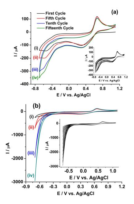
**Fig. 7** Cyclic voltammograms of (U, Pu)C FBTR fuel sample on (a) rGO/GC and (b) GC electrodes at a scan rate of 50 mV s<sup>-1</sup> for (i) first, (ii) fifth, (iii) tenth and (iv) fifteenth cycle. The insets show the continuous cyclic voltammograms of 15 cycles.
