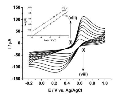
**Fig. 3** Cyclic voltammograms of 10 mM Pu(IV) in 1 M  $H_2SO_4$  solution on rGO/GC electrodes at a scan rate (v) of (i) 10, (ii) 25, (iii) 50, (iv) 75, (v) 100, (vi) 150, (vii) 200 and (viii) 250 mV s<sup>-1</sup>. The inset shows the plots of Ln (I<sub>p</sub>) versus Ln (v) for (1) cathodic and (2) anodic peaks.
