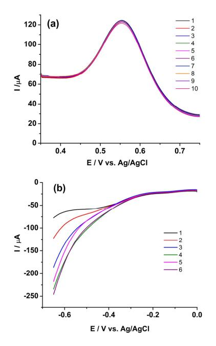
**Fig. 6** Square wave voltammograms of (U, Pu)C FBTR sample on rGO/GC for (a) anodic scan from 0.35 V to 0.75 V for analyzing Pu and (b) cathodic scan from 0 V to -0.65 V for analyzing U. Square wave amplitude = 25 mV; Square wave frequency = 20 Hz; Step potential increment = 1 mV; Standby time at 0.35 V (for a) and at 0 V (for b) is 10 s. The numeric represents the sequence of the replicate measurements.
