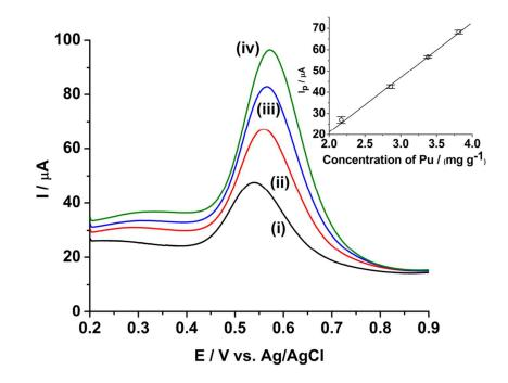
**Fig. 5** ASWVs of (i) 2.17, (ii) 2.86, (iii) 3.38 and (iv) 3.81 mg g<sup>-1</sup> of Pu in 1 M H<sub>2</sub>SO<sub>4</sub> on rGO/GC. Square wave amplitude = 25 mV; Square wave frequency = 20 Hz; Step potential increment = 1 mV; Hold time at initial potential = 10 s. Inset shows the sensitivity plot for the same. The vertical bars shown in the inset represent the standard deviation ( $\sigma$ ) of I<sub>p</sub> obtained from ten replicate measurements for each concentration of Pu.
