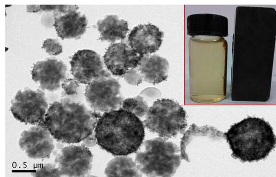
Fig. 9 TEM images of magnetic PAA microgels prepared with the weight ratio of AN/DVB/MPS-Fe<sub>3</sub>O<sub>4</sub>/HD = 15.0/1.8/1.5/0.80 (Sample 12 in Table 1). Photo of the magnetic microgels under magnetic field was
