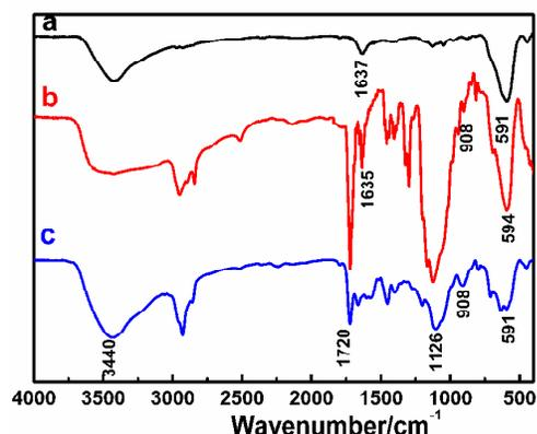
**Fig. 4** FTIR spectra of  $\text{Fe}_3\text{O}_4$  nanoparticles (a), MPS- $\text{Fe}_3\text{O}_4$  nanoparticles (b) and  $\text{Fe}_3\text{O}_4$ /PAA hybrid microgels (c).
