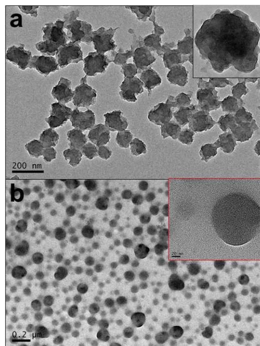
**Fig. 6** TEM images of PAN nanoparticles prepared with 1.8 g of DVB (a) and PAA nanogels (b). Insets show the corresponding high-resolution TEM image.
