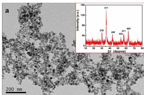
**Fig. 1** TEM image of magnetic nanoparticles. Inset shows the XRD pattern of magnetic nanoparticles.
