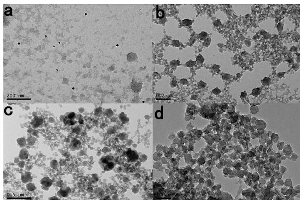
**Fig. 5** TEM images of PAN nanoparticles prepared with 0.6 g (a), 0.9 g
