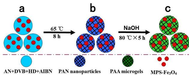
**Scheme 1** Illustration for the preparation of magnetic PAA nanogels *via* miniemulsion polymerization.
