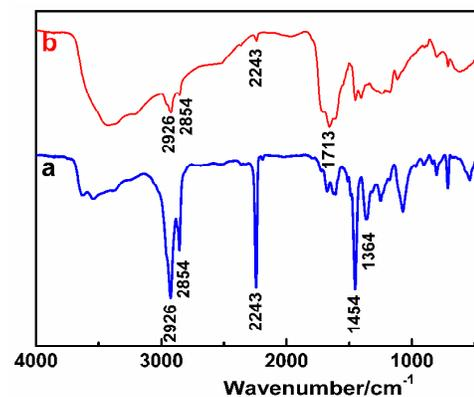
**Fig. 3** FTIR spectra of PAN nanoparticles (a) and PAA nanogels (b).
