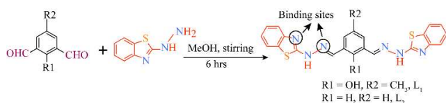
Scheme 1. Synthetic scheme of the receptors with the binding sites for guest metals.
