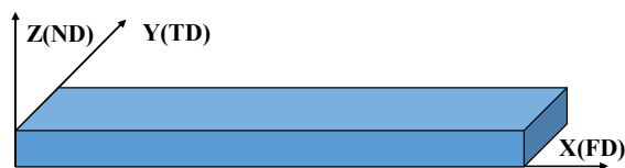
Fig.1 Definition of the direction, X is the flow direction denoted as FD, Y is the transverse direction denoted as TD and Z is the normal direction denoted as ND.
