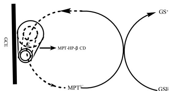
Scheme 2. Reaction scheme for the electrocatalytic oxidation of GSH.
