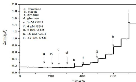
Fig. 10. Amperometric response of MPT-HP- $\beta$ CD/GCE to sequential additions of fructose, starch, glycine, glucose and various concentration of GSH into stirring 0.1 M PBS (pH 7.0) at an applied potential of 0.6 V vs. Ag/AgCl.
