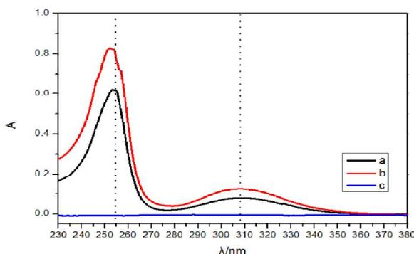
Fig. 2. UV-visible absorption spectra recorded of (a) MPT, (b) MPT-HP- $\beta$ CD, (c) HP- $\beta$ CD.
