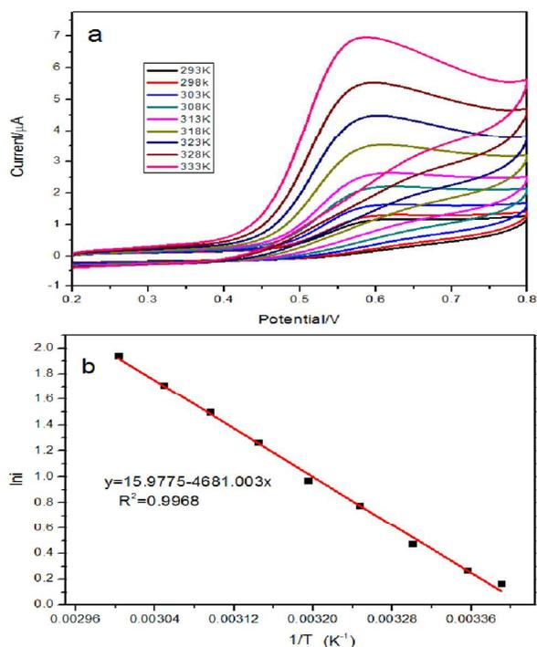
Fig. 8. (a) CVs of MPT-HP-βCD/GCE in 9.7 μM GSH + 0.1 M PBS solution under different temperature. (b) Display the logarithm plots of peak current against the reciprocal of temperature.
