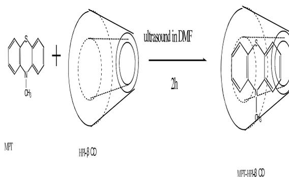
Scheme 1. Schematic illustrates the reaction steps of MPT-HP- $\beta$ CD
