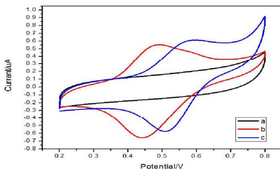
Fig. 4. CVs of (a) GCE, (b) MPT/GCE and (c) MPT-HP-βCD/GCE in 0.1 M PBS solution (pH=7.0)
