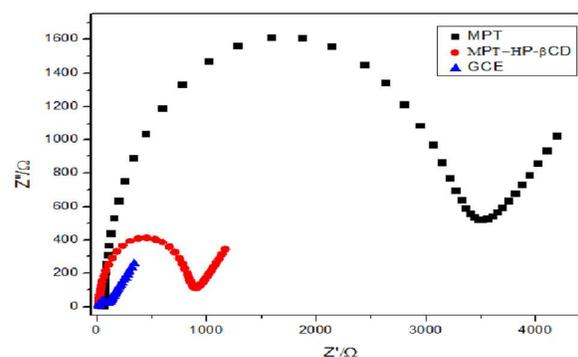
Fig. 3. Nyquist plots of GCE (blue), MPT/GCE (black) and MPT-HP- $\beta$ CD/GCE (red) electrodes in the presence of  $0.1\text{ mM K}_3\text{Fe}(\text{CN})_6/\text{K}_4\text{Fe}(\text{CN})_6$  with  $0.1\text{ M KCl}$  solution. The potential applied to the electrode was the open circuit voltage of this test system ( $0.2210\text{ V vs. Ag/AgCl}$ ).
