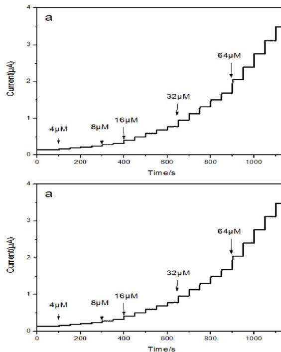
Fig. 9. (a) Amperometric current versus time (*i-t*) curve for the detection of GSH at MPT-HP-βCD/GCE at 0.58 V. GSH was successively injected into the stirred 0.1 M pH 7.0 PBS with 4 μM, 8 μM, 16 μM, 32 μM, 64 μM. (b) The calibration plot of the GSH biosensor.
