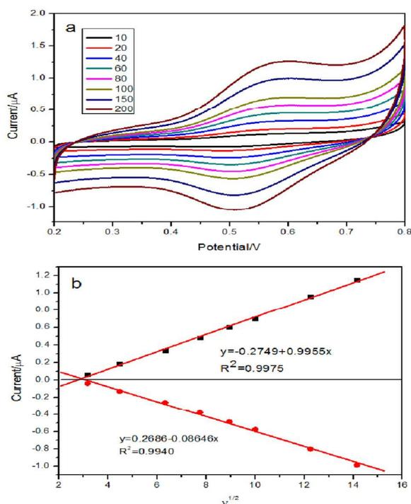
Fig.6. (a) CVs of MPT-HP- $\beta$ CD / GCE in 0.1 M PBS solution (pH=7.0) at different scan rate (10–200 mV/s). (b) Display the plots of peak current against square root of scan rate.
