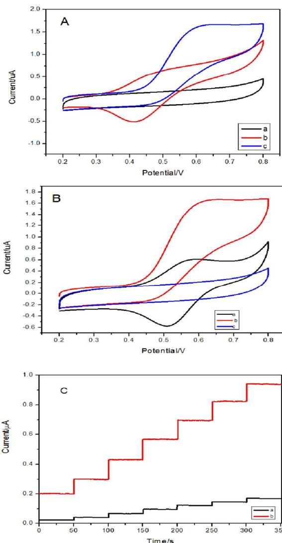
Fig. 5. (A) CVs of (a) GCE, (b) MPT/GCE, (c) MPT-HP-βCD / GCE in 9.7  $\mu$ M GSH + 0.1 M PBS solution (pH=7.0). (B) CVs of (a) MPT-βCD / GCE in 0.1 M PBS solution without GSH, (b) MPT-βCD / GCE in 0.1 M PBS solution with 9.7  $\mu$ M GSH, (c) GCE in 0.1 M PBS solution with 9.7  $\mu$ M GSH. (C) Chronoamperometric responses of 16  $\mu$ M GSH at MPT/GCE (a), MPT-HP-βCD (b) electrode, potential applied: 0.58V (vs. Ag/AgCl).
