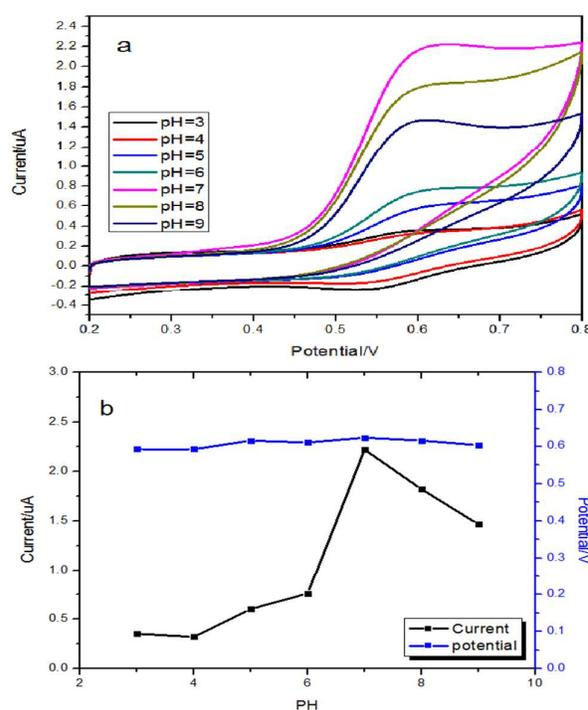
Fig.7. (a) CVs of MPT-HP- $\beta$ CD/GCE in 9.7  $\mu$ M GSH + 0.1 M PBS solution at different pHs (3–9). (b) Display the plots of peak current (black) and Potential (blue) against pHs.
