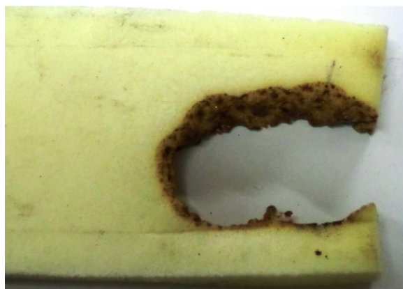
Figure 5. Burnt virgin PU foam
