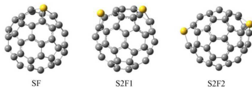
Fig. 1 The optimized structures of Mono and disulfur-doped fullerene as employed adsorbents in the calculations
