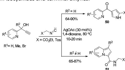
**Scheme 30** Synthesis of indolizines and 2,4-disubstituted pyrroles.
