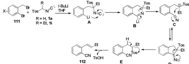
**Scheme 69** Proposed mechanism for the isocyanide-cyanide rearrangement.
