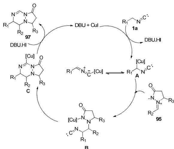
Scheme 62 Mechanism for the synthesis of 1,2,4-triazines.
