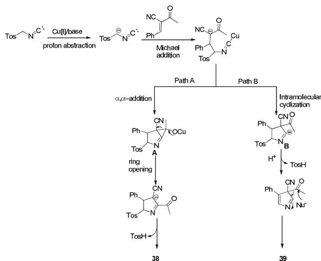
**Scheme 21** Mechanistic route for the synthesis of fused 2-acylpyrroles.
