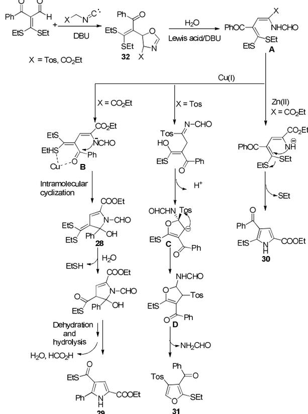
**Scheme 16** Proposed mechanism for the synthesis of various annulated pyrroles.
