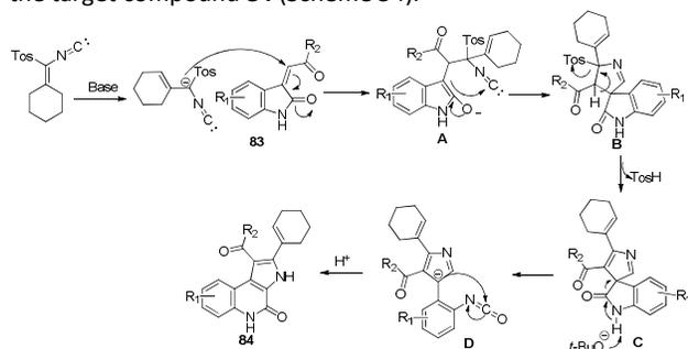
**Scheme 54** Mechanism for the synthesis of 3H-pyrrolo[3,2-c]quinolinones.
