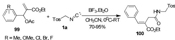
Scheme 63 Synthesis of trisubstituted olefins derivatives.
