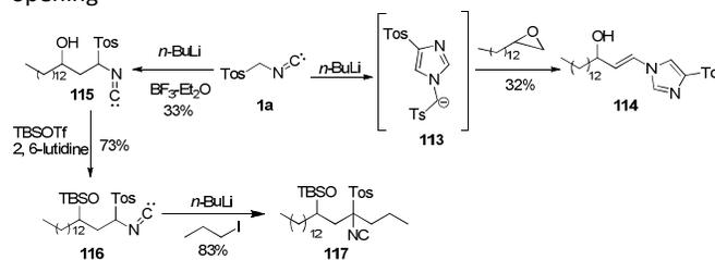
**Scheme 70** Synthesis of hydroxyl derivatives *via* TosMIC mediated epoxide ring opening.
