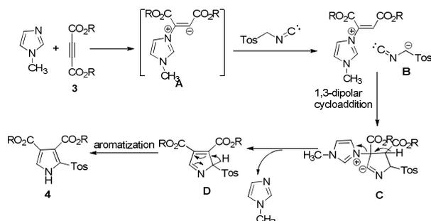
**Scheme 4** Proposed mechanism for the substituted pyrrole-3,4-dicarboxylates.
