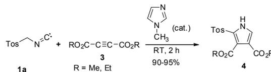
**Scheme 3** Synthesis of dialkyl 2-[(4-methylphenyl) sulfonyl]-1*H*-pyrrole-3,4-dicarboxylates.
