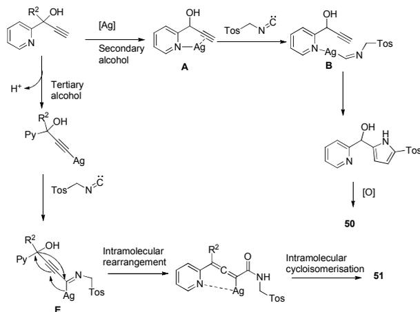
**Scheme 31** Plausible reaction mechanism to synthesize indolizines and 2,4-disubstituted pyrroles.
