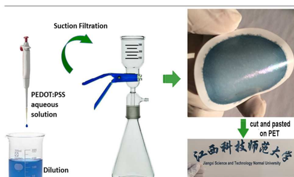
Fig. 1 Schematic illustration of suction filtration for PEDOT:PSS thin-film on PVDF.
