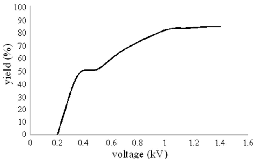
Figure 4. The yield of biodiesel synthesis versus the applied voltage.
