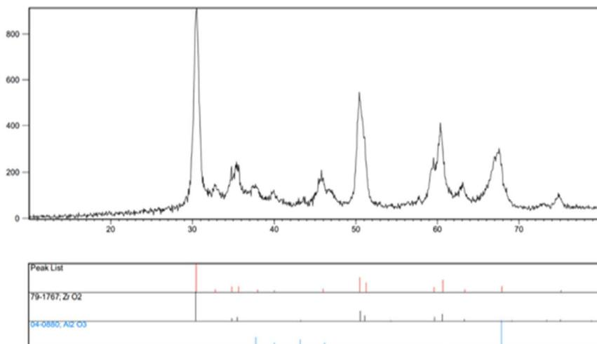
Figure 2. XRD pattern of  $ZrO_2/Al_2O_3$  nano-catalyst
