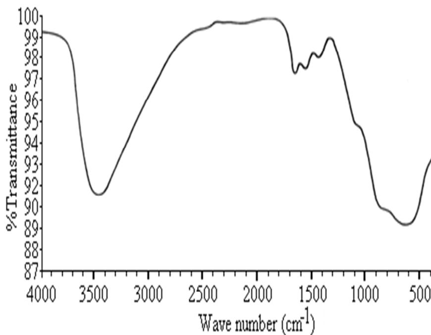
Figure 3. FTIR spectrum of  $ZrO_2/Al_2O_3$  nano-catalyst
