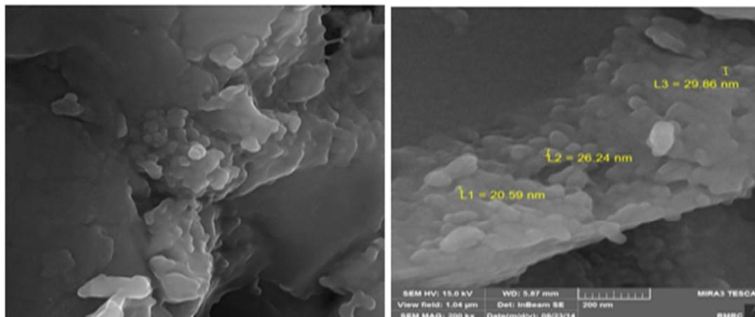
Figure 1. FESEM image of  $\text{ZrO}_2/\text{Al}_2\text{O}_3$  nano-catalyst
