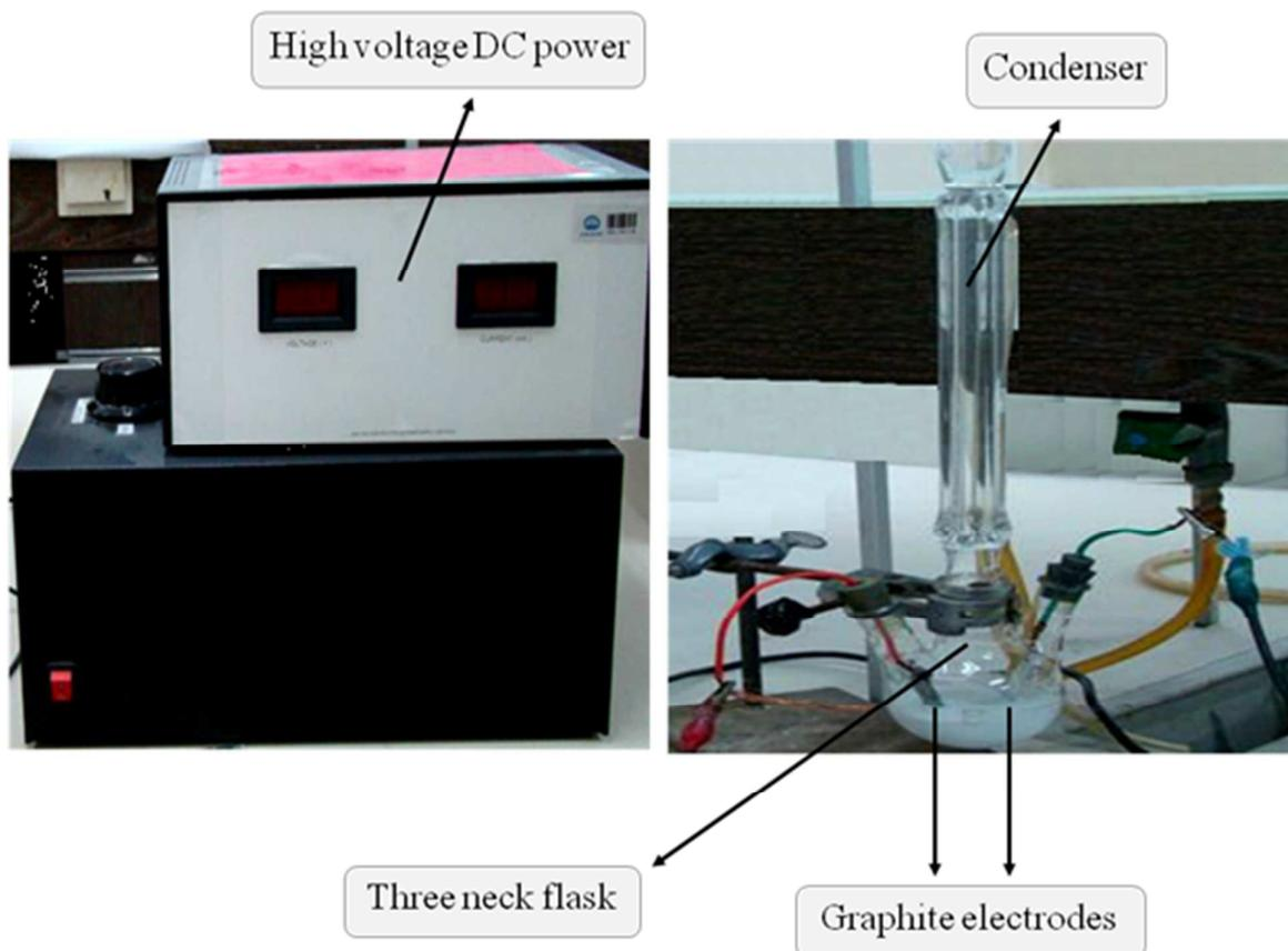
Figure 5. The High voltage esterification apparatus.
