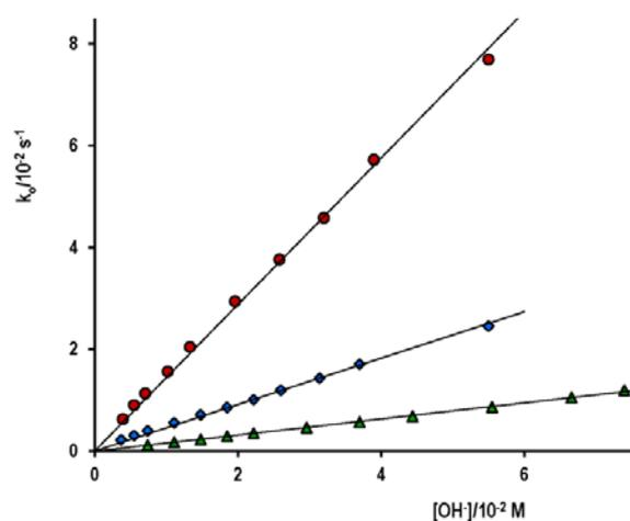
Figure 1. Plot of the observed rate constant,  $k_o$ , for the alkaline hydrolysis of (●)PhA, (◆)PhB and (▲)ASA as a function of the OH<sup>-</sup> concentration, ionic strength 0.10 M and 25 °C.
