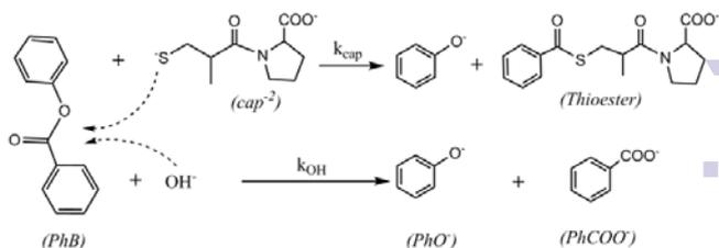
**Scheme 2.** Reaction paths of PhB cleavage in aqueous basic medium in the presence of captopril.
