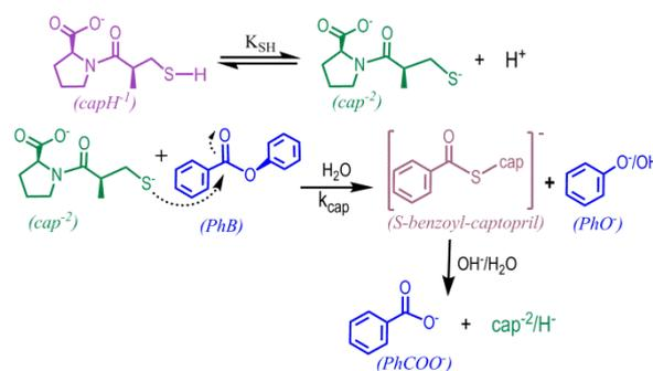
**Scheme 3.** Proposed reaction steps in aqueous buffered solution of CO<sub>3</sub><sup>2-</sup>/CO<sub>3</sub>H<sup>-</sup>.
