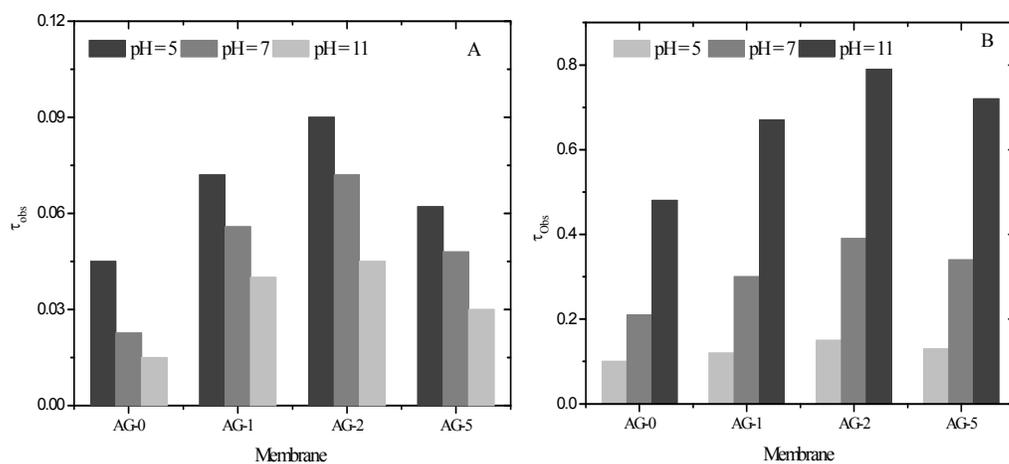
**Fig. 10.** The observed transmission ( $\tau_{obs}$ ) for: (A) BSA and (B) LYZ ( $1 \text{ g L}^{-1}$ ) through positively charged hybrid membranes at varied  $pH$ , 1 bar applied transmembrane pressure and a stirring speed of 400 rpm.
