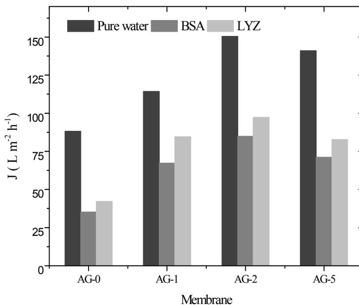
**Fig. 7.** Pure water flux and protein (BSA and LYZ) solution flux for positively charged hybrid membranes at varied fraction of GO nanosheets (%), 1 bar applied pressure,  $pH = 7$  and a stirring speed of 400 rpm.
