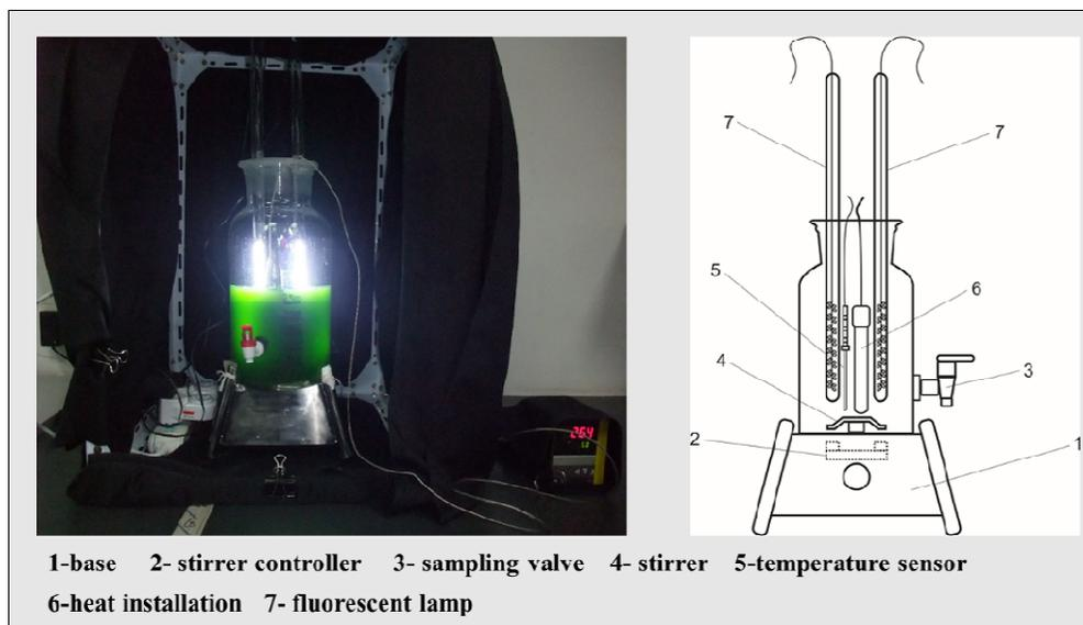
**Fig.1.** The set-up diagram of the algal reactor in the present study.
