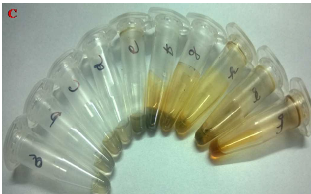
Figure S1. Formation of AgNPs as a function of: (C) 3-APTMS concentrations (Table S1C, Sr. no. a to j) keeping constant concentrations of Formaldehyde (0.8 M) and 0.01 M AgNO 3 .
