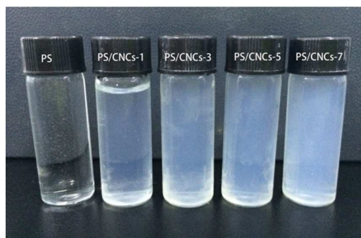
Fig.3. Photograph of spinning solutions with various CNC contents
