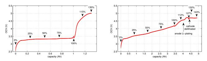
**Fig. 1** OCV characteristics of the (left) LFP and (right) NCA cells. Measured values in the allowed voltage range and additionally in the overcharge region are given. SOC points, at which temperature-ramp experiments were done, are marked. Rough estimates, where Li-plating and complete cathode delithiation may occur, are indicated for the NCA cell. The discontinuities at 100% are caused by relaxations during the time-gaps between cycling and the overcharge experiments.
