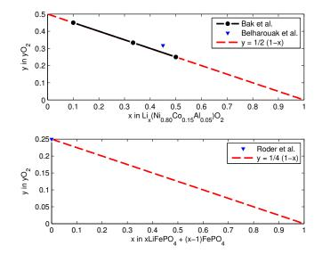
**Fig.** 6 Oxygen release at different lithiation states: (a) NCA powder upon heating up to  $600^{\circ}$ C (from<sup>59,61</sup>) and (b) LFP powder in electrolyte upon heating to  $350^{\circ}$ C (from<sup>64</sup>).
