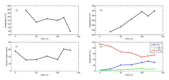
Fig. 5 Summary of all experiments with LFP cells at different SOC: (a) Onset cell temperature  $\theta_o$ . (b) Maximum cell temperature  $\theta_m$ . (c) amount of produced gas  $n_{sum}^{ideal}$ . (d) main detected gas components  $r_i^{GC}$ .
