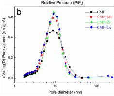
Fig. 1 (a) The  $N_2$  physisorption isotherms and (b) the pore significant distribution patterns of the CMF catalysts with different additives
