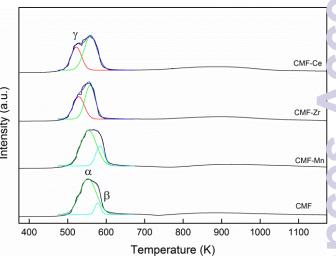
Fig. 5 H<sub>2</sub>-TPR profile of the CMF-M catalysts with different additives
