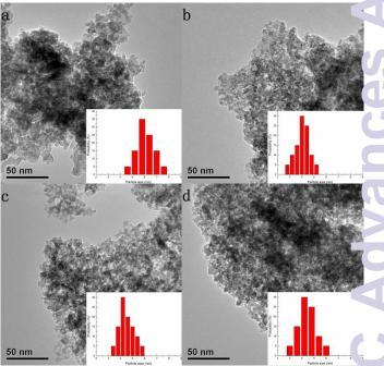
Fig. 3 TEM images of the CMF-M catalysts with different additives (a, CMF; b, CMF-Mn; c, CMF-Zr; d, CMF-Ce)
