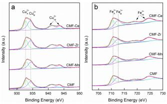
Fig. 4 XPS spectra of the (a) Cu 2p and (b) Fe 2p regions in the CMF-M (M=Mn, Zr, Ce) catalysts
