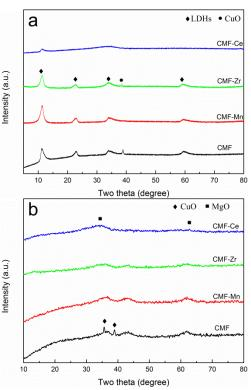
Fig. 2 XRD patterns of the as-synthesized catalysts (a) before and (b) after calcination
