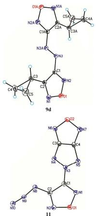
55 Fig.4 General view of the structures 9d and 11 with the atom numbering scheme. Displacement ellipsoids are drawn at the 50% probability level.
