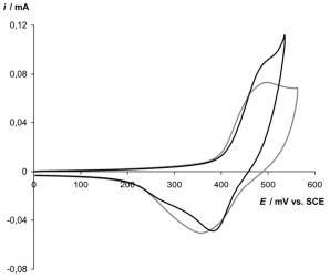
**Figure 2**. CVs of Ni/NiOOH in 0.2 M NaOH with (black dotted line) and without (gray solid line) amine **8a** (20 <sup>70</sup> mmol L<sup>-1</sup>, 100 mV s<sup>-1</sup>).
