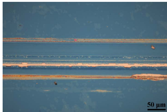
Figure 7. Optical microscopy image of the wear track for ZnO film deposited at 150 °C under normal load of 0.5 N.
