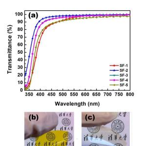
**Fig. 5** (a) UV-Vis spectra of the  $PI_{6FDA-APB(Si)}$ \_SiO<sub>2</sub>-20% binary composite (SF-1), and  $PI_{6FDA-APB(Si)}$ \_HBP $I_{BPADA-TAP(OH)}$ -10~40%\_SiO<sub>2</sub>-20% ternary 25 hybrid composites (SF-2~5). The film thickness was under 10  $\mu$ m on the glass substrates. (b) commercial Kapton film (25  $\mu$ m) and (c) SF-2 film (28  $\mu$ m).
