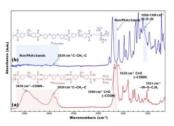
10 Fig. 2 FTIR spectra of (a) the silica terminated polyamic acids (PAA<sub>6FDA</sub>-APB(Si) in NMP solvent, and (b) PI<sub>6FDA-APB(Si)</sub>\_SiO<sub>2</sub>-20% binary composite (SF-1).
