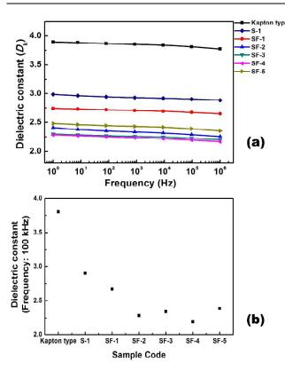
Fig. 3 Dielectric constant (Dk) of the PI<sub>6FDA-APB</sub> unary PI (S-1), PI<sub>6FDA-APB</sub> APB(Si)\_SiO<sub>2</sub>-20% binary composite (SF-1), and PI(Si)\_HBPI(OH)-10~40%\_SiO<sub>2</sub>-20% hybrid ternary composites (SF-2~5); (a) scanning 5 frequency from 1 Hz to 10<sup>6</sup> Hz, (b) fixed frequency of 100 kHz.
