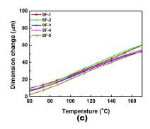
Fig. 6 (a) DSC, (b) TGA, and (c) CTE curves for the PI<sub>6FDA-APB(Si)</sub>\_SiO<sub>2</sub>-20% (SF-1) binary composite, and PI<sub>6FDA-APB(Si)</sub>\_HBPI<sub>BPADA-TAP(OH)</sub>-5 10~40% SiO<sub>2</sub>-20% ternary hybrid composites (SF-2~5).
