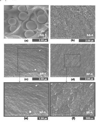
Fig. 4 Typical SEM images of PI and the composites, (a)  $PI_{6FDA-APB}\_SiO_2-20\%$  (SA-1), <sup>23</sup> (b)  $PI_{6FDA-APB}\_HBPI_{BPADA-TAP(OH)}-30\%\_SiO_2-20\%$  (SA-4), <sup>23</sup> 55 (c), (e)  $PI_{6FDA-APB(Si)}$ SiO<sub>2</sub>-20% (SF-1), and (d), (f)  $PI_{6FDA-APB(Si)}$  $_{APB(Si)}$ \_HBPI $_{BPADA\text{-}TAP(OH)}$ -30%\_SiO $_{2}$ -20% (SF-4); Scale bar: 2  $\mu m$  (a-d), 1 μm (e), and 500 nm (f). Pictures from reference 23 are reproduced with permission.
