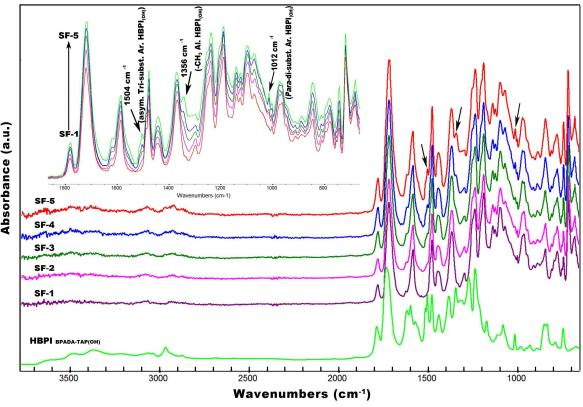
Fig. 1 FTIR spectra of the hydroxyl terminated hyperbranched polyimide, PI<sub>0FDA-APB(Si)</sub>\_SiO<sub>2</sub>-20% binary composite (SF-1), and PI<sub>(Si)</sub>\_HBPI<sub>(OH)</sub>-10~40%\_SiO<sub>2</sub>-20% hybrid ternary composites (SF-2~5).
