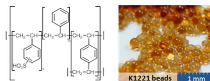
Figure 1. Chemical structure of the K1221 ion exchange resin (left) and image of the parent K1221 beads (right).
