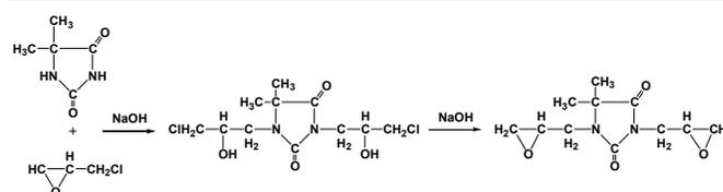
Fig. 1 The reaction equation of the DMHP.
