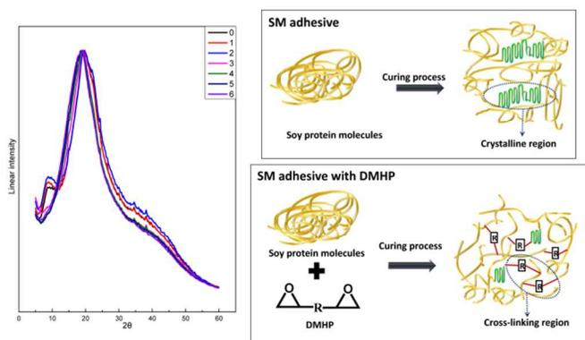
Fig. 7 The X-ray diffraction patterns of different adhesive samples: 0 (SM adhesive), 1 (SM/PAM adhesive), 2 (SM/PAM/SDS adhesive), 3 (SM/PAM/SDS/DMHP-5 wt% adhesive), 4 (SM/PAM/SDS/DMHP-9 wt% adhesive), 5 (SM/PAM/SDS/DMHP-13 wt% adhesive), 6 (SM/PAM/SDS/DMHP-17 wt% adhesive). And the effect of DMHP on adhesive crystallinity reduction.
