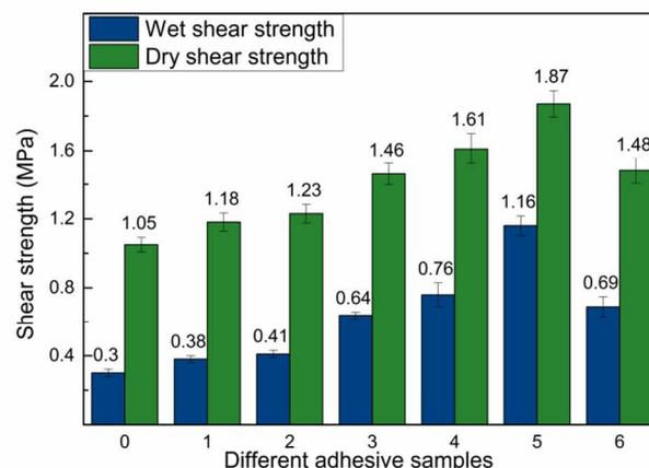
**Fig. 3** The wet/dry shear strength of the plywood bonded by different adhesive samples: 0 (SM adhesive), 1 (SM/PAM adhesive), 2 (SM/PAM/SDS adhesive), 3 (SM/PAM/SDS/DMHP-5 wt% adhesive), 4 (SM/PAM/SDS/DMHP-9 wt% adhesive), 5 (SM/PAM/SDS/DMHP-13 wt% adhesive), 6 (SM/PAM/SDS/DMHP-17 wt% adhesive).
