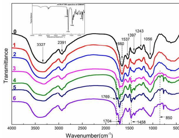
**Fig. 5** FTIR spectra of of different adhesive samples: 0 (SM adhesive), 1 (SM/PAM adhesive), 2 (SM/PAM/SDS adhesive), 3 (SM/PAM/SDS/DMHP-5 wt% adhesive), 4 (SM/PAM/SDS/DMHP-9 wt% adhesive), 5 (SM/PAM/SDS/DMHP-13 wt% adhesive), 6 (SM/PAM/SDS/DMHP-17 wt% adhesive). And the curing process of the SM/PAM/SDS/DMHP adhesive.
