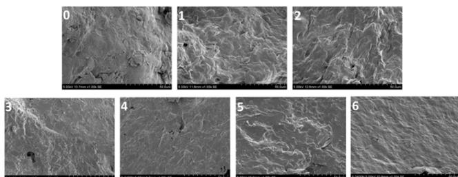
**Fig. 9** The fracture surface micrograph of different cured adhesive samples: 0 (SM adhesive), 1 (SM/PAM adhesive), 2 (SM/PAM/SDS adhesive), 3 (SM/PAM/SDS/DMHP-5 wt% adhesive), 4 (SM/PAM/SDS/DMHP-9 wt% adhesive), 5 (SM/PAM/SDS/DMHP-13 wt% adhesive), 6 (SM/PAM/SDS/DMHP-17 wt% adhesive).
