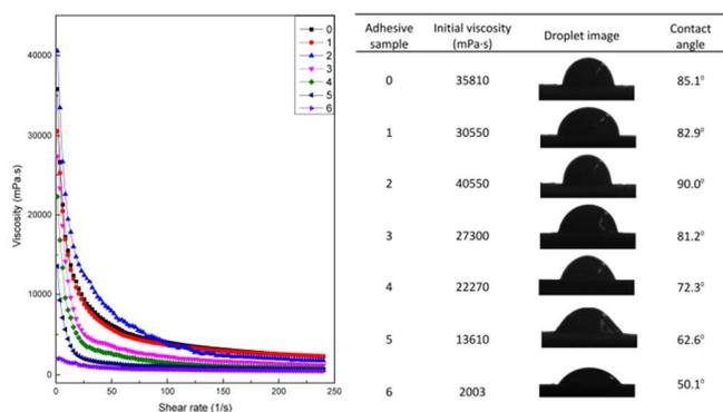
**Fig. 4** The droplet picture on the wood substrate in 5 s after the deposition and apparent viscosity of different adhesive samples: 0 (SM adhesive), 1 (SM/PAM adhesive), 2 (SM/PAM/SDS adhesive), 3 (SM/PAM/SDS/DMHP-5 wt% adhesive), 4 (SM/PAM/SDS/DMHP-9 wt% adhesive), 5 (SM/PAM/SDS/DMHP-13 wt% adhesive), 6 (SM/PAM/SDS/DMHP-17 wt% adhesive).
