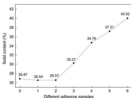
**Fig. 2** The solid content of different adhesive samples: 0 (SM adhesive), 1 (SM/PAM adhesive), 2 (SM/PAM/SDS adhesive), 3 (SM/PAM/SDS/DMHP-5 wt% adhesive), 4 (SM/PAM/SDS/DMHP-9 wt% adhesive), 5 (SM/PAM/SDS/DMHP-13 wt% adhesive), 6 (SM/PAM/SDS/DMHP-17 wt% adhesive).
