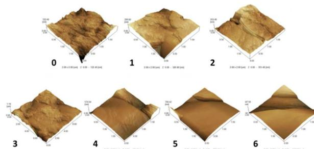
Fig. 8 AFM 3-dimensional image of different cured adhesive samples: 0 (SM adhesive), 1 (SM/PAM adhesive), 2 (SM/PAM/SDS adhesive), 3 (SM/PAM/SDS/DMHP-5 wt% adhesive), 4 (SM/PAM/SDS/DMHP-9 wt% adhesive), 5 (SM/PAM/SDS/DMHP-13 wt% adhesive), 6 (SM/PAM/SDS/DMHP-17 wt% adhesive).
