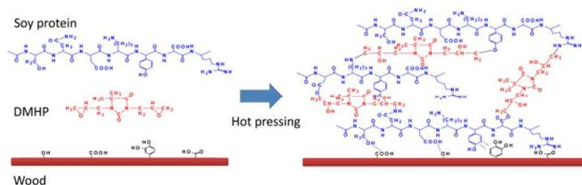
Fig. 6 The curing process of the SM/PAM/SDS/DMHP adhesive.
