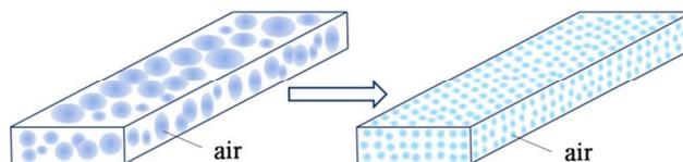
Fig. 3 Schematic images of the microstructure's change of the adhesion material with the growth of the amount of the foam stabilizer. The circles represent air bubbles.
