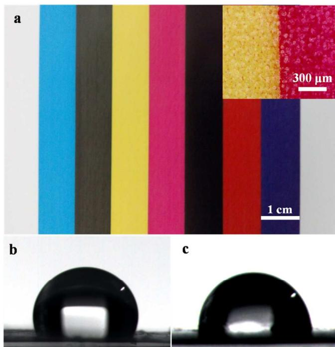
**Fig. 6** The porous material (5 wt% of ammonium stearate) printed with color piece (a), and the contact angle of the porous material before (b) and after (c) digital inkjet printing
