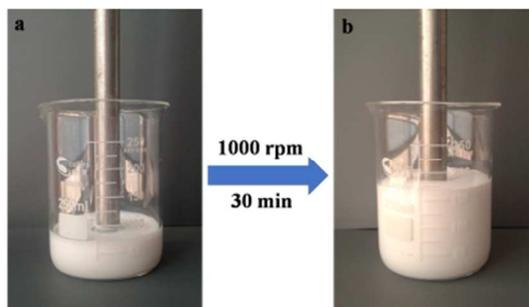
Fig. 1 Images of PBA emulsion with foam stabilizer before (a) and after (b) stirred. (The amount of ammonium stearate emulsion was 5 wt %)
