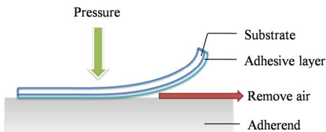
Fig. 5 Schematic image of adhesion process of porous material (The substrate was PP, the adhesive layer was porous polymer, and the adherend could be stainless steel, glass and aluminium)
