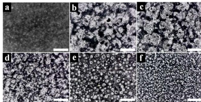
Fig. 2 Microscope photographs of obtained adhesion materials with pores using foamed emulsion with different amounts of foam stabilizer. (a. 0 %, b. 1 wt %, c. 2 wt %, d. 3 wt %, e. 4 wt %, f. 5 wt %). The scale bars equal 300  $\mu$ m.
