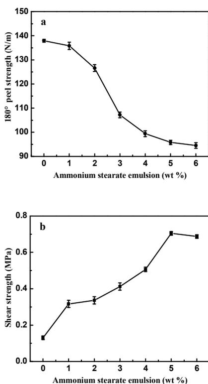
Fig. 4 Effect of the amount of ammonium stearate emulsion on 180° peel strength (a) and shear strength (b)
