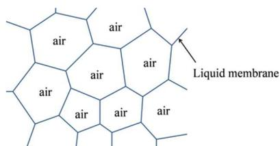
Scheme 1 Illustration of liquid membrane
