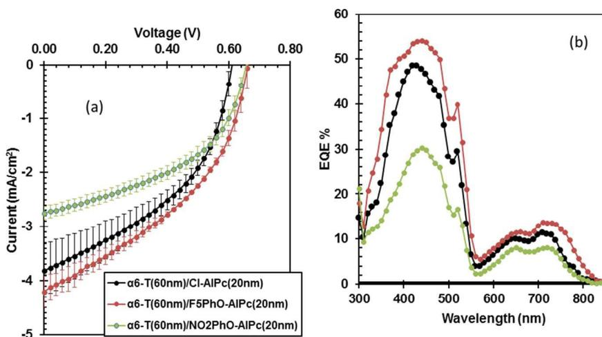
**Figure 6.** (a) The average J-V curves and (b) the average external quantum efficiencies of α-6T/Cl-AIPc, and α-6T/F<sub>5</sub>PhO-AIPc, and α-6T/NO<sub>2</sub>PhO-AIPc OPVs.
