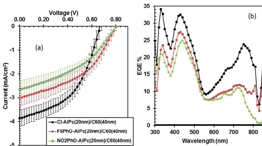
**Figure 5.** (a) The average J-V curves and (b) the average external quantum efficiencies of Cl-AIPc /C<sub>60</sub>, F<sub>5</sub>PhO-AIPc/C<sub>60</sub>, and NO<sub>2</sub>PhO-AIPc/C<sub>60</sub> OPVs.
