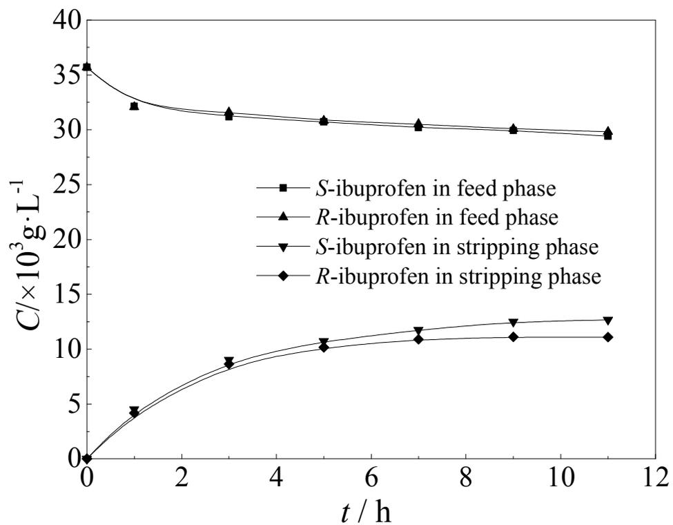
**Fig. 2** Changes of ibuprofen enantiomers concentration via time in feed and stripping phases.
