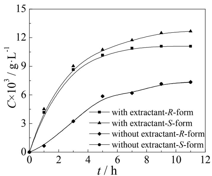
**Fig. 3** The concentration of ibuprofen enantiomers in stripping phase with and without chiral extractant in membrane phase.
