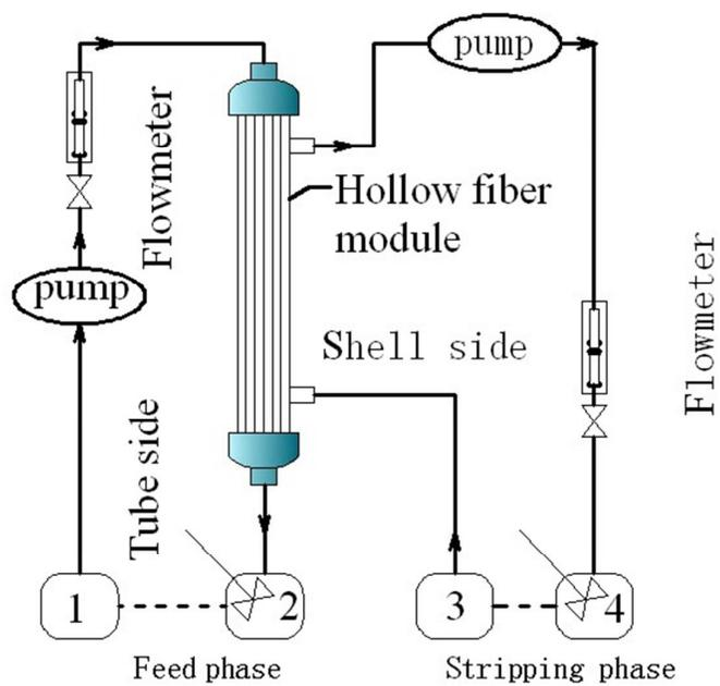
**Fig. 1** Flow diagram of enantioselective separation of racemic ibuprofen by chiral liquid membrane.
