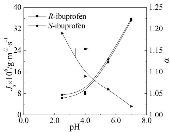
**Fig. 10** Influence of pH in stripping phase on mass transfer flux in stripping phase and separation factor in chiral liquid membrane process.
