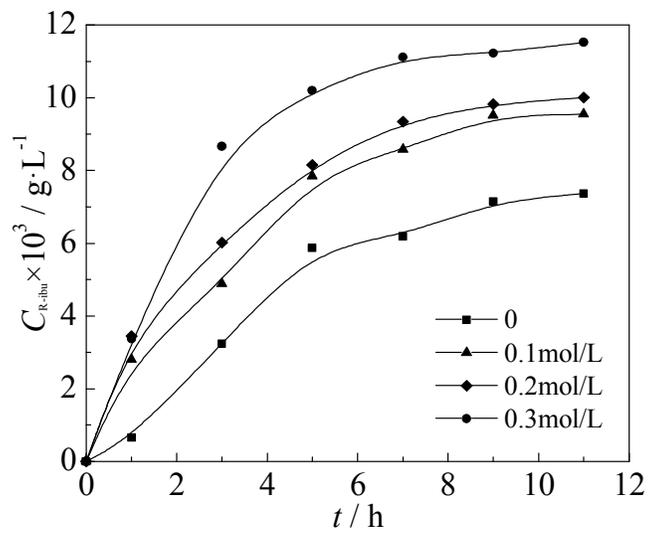
**Fig. 5** Influence of concentration of *L*-dipentyl tartrate ester in the membrane phase on the concentration of R-ibuprofen in stripping phase.
