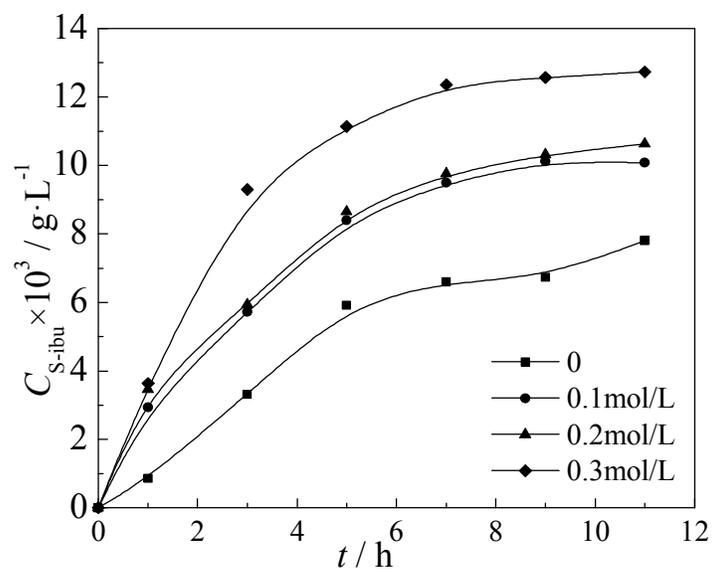
**Fig. 6** Influence of concentration of *L*-dipentyl tartrate in the membrane phase on the concentration of *S*-ibuprofen in stripping phase.
