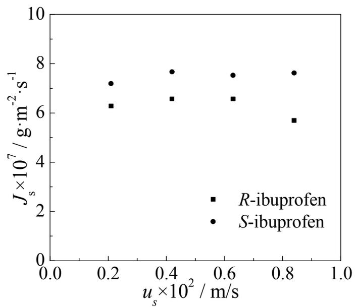
**Fig. 9** Influence of flow rates of shell side on mass transfer flux in stripping phase.
