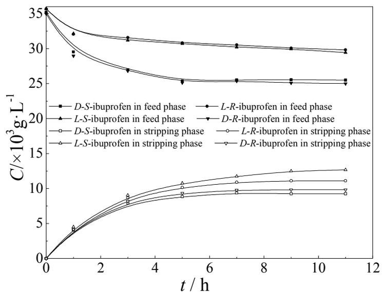
**Fig. 4** The concentration of ibuprofen enantiomers via time in feed and stripping phases with different types of chiral extractants in membrane phase.
