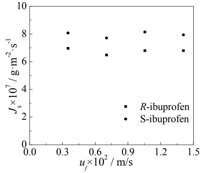
**Fig. 8** Influence of flow rates of tube side on mass transfer flux in stripping phase.
