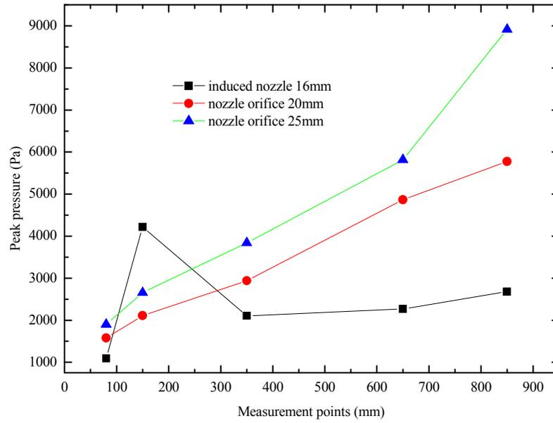
Fig.11 peak pressures over the full height of filter cartridge with three different nozzles (induced nozzle  $\Phi$ 16 mm with jet distance 60 mm, nozzle  $\Phi$ 20 mm with 280 mm, nozzle  $\Phi$ 25 mm with jet distance 200 mm)
