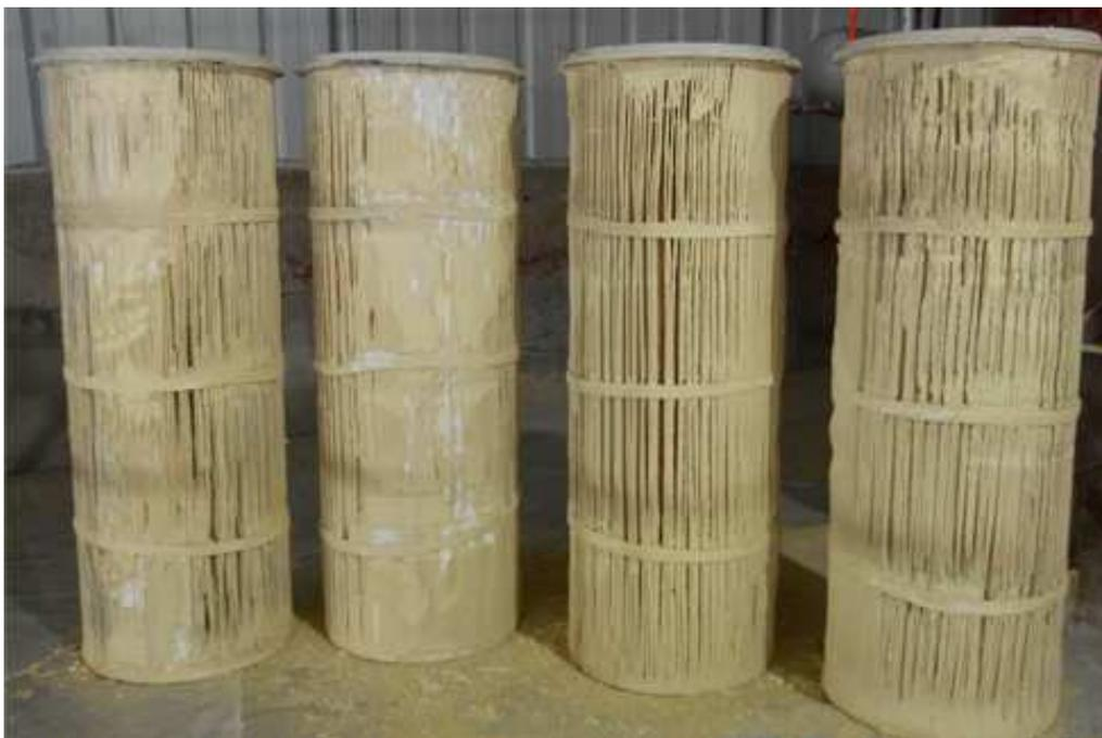
Fig.1 Difficult cleaning of pleated filter cartridges for collecting pesticide particles (with induced nozzle  $\Phi 16\text{mm}$ , the filter cartridges are taken out the filters after the operational time 60 min)
