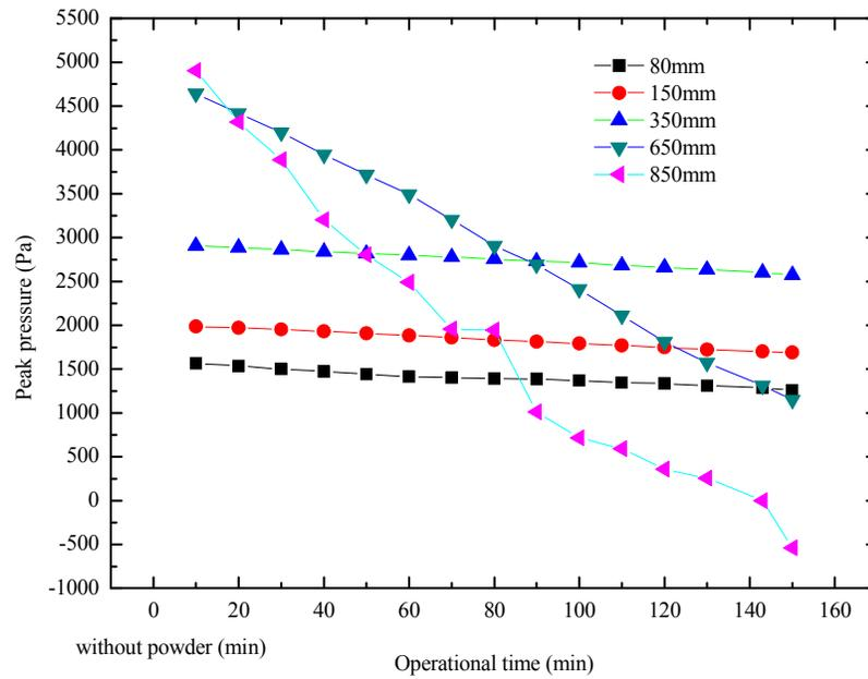
Fig.16 effect of operational time on peak pressure with the nozzle orifice  $\Phi 20$  mm
