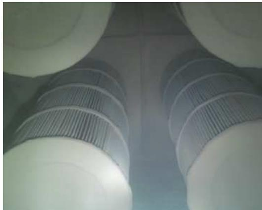
Fig.14 Bottom of filter cartridge filled with dust particles resolved using the nozzle  $\Phi 25$  mm (views from the bottom after operational time 180 min)
