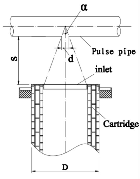
Fig.10 the relative of nozzle orifice and jet distance
