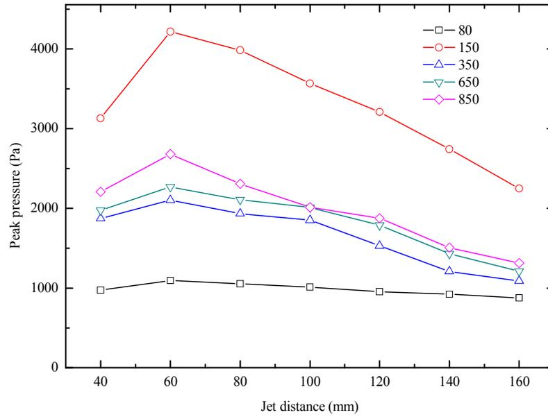
Fig.7 effect of jet distance on peak pressure with the induced nozzle  $\Phi 16$  mm
