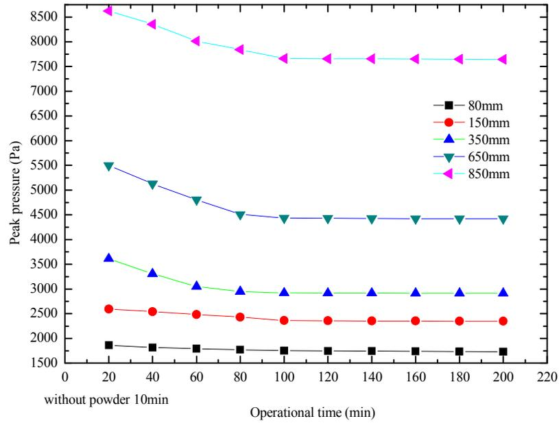
Fig.17 effect of operational time on peak pressure with the nozzle orifice  $\Phi 25$  mm
