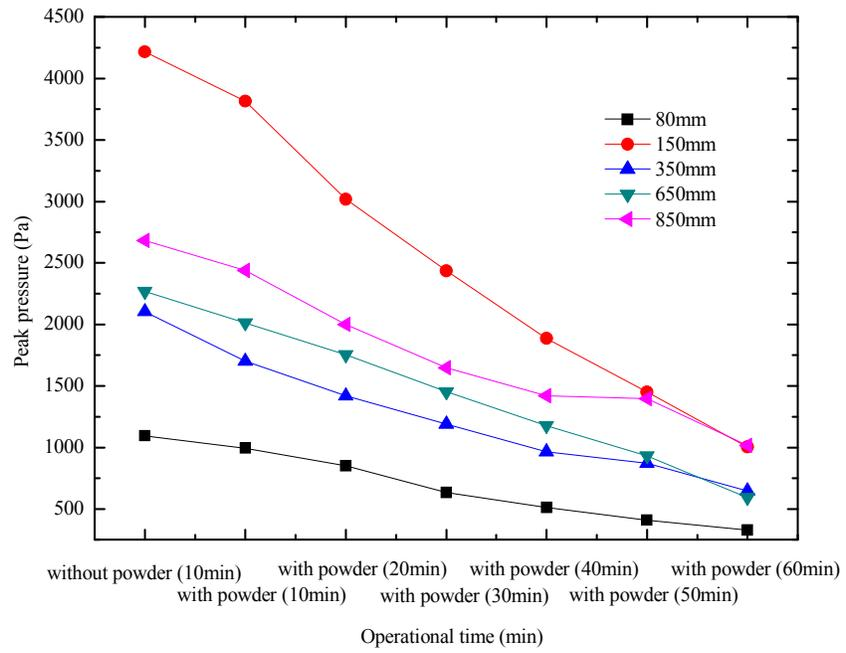
Fig.15 effect of operational time on peak pressure with the induced nozzle  $\Phi 16$  mm
