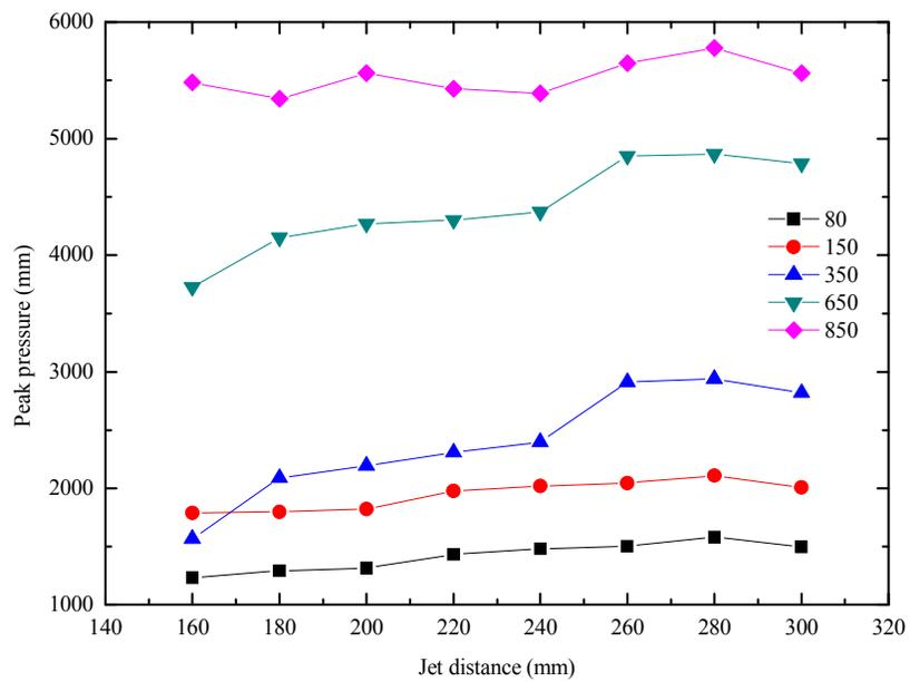
Fig.8 effect of jet distance on peak pressure with the nozzle orifice  $\Phi 20$  mm
