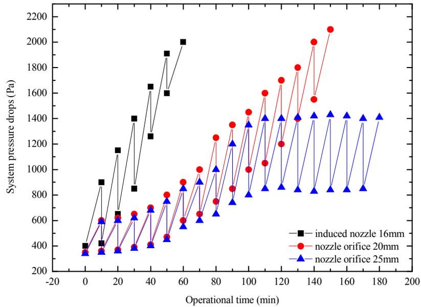
Fig.12 systematic pressure drops vs operational time during clogging/cleaning cycles
