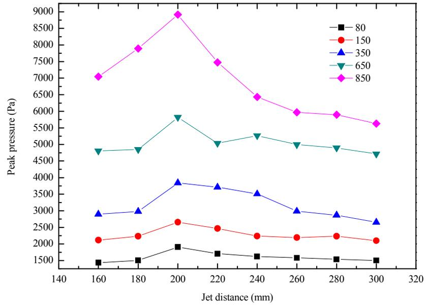
Fig.9 effect of jet distance on peak pressure with the nozzle orifice  $\Phi 25$  mm
