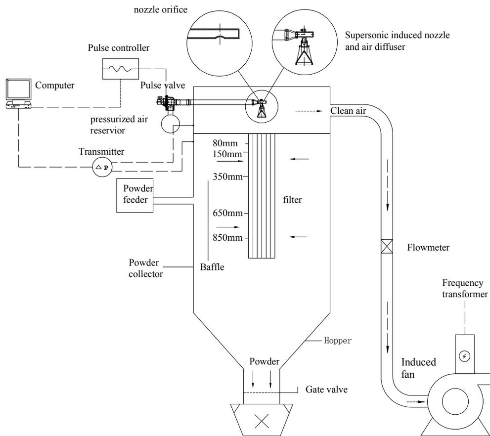
Fig.2 Schematic view of the test rig
