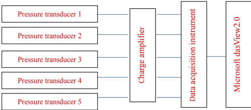
Fig.6 the systematic connection method
