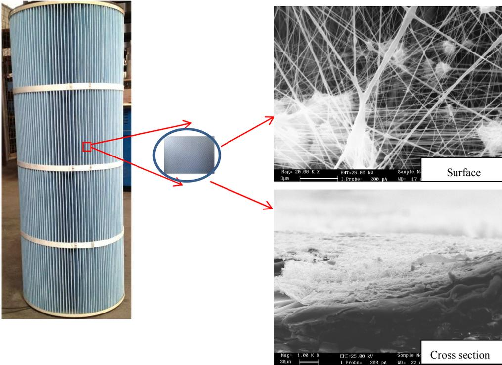
a. photo of filter cartridge and microstructure of filter medium
