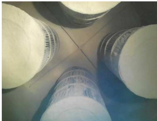
Fig.13 Bottom of filter cartridge filled with dust particles using the nozzle  $\Phi 20$  mm (views from the bottom after operational time 150 min)
