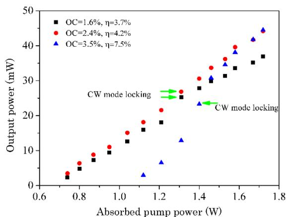
Fig. 3. Average output power versus absorbed pump power of the mode-locked laser using three different output couplers.
