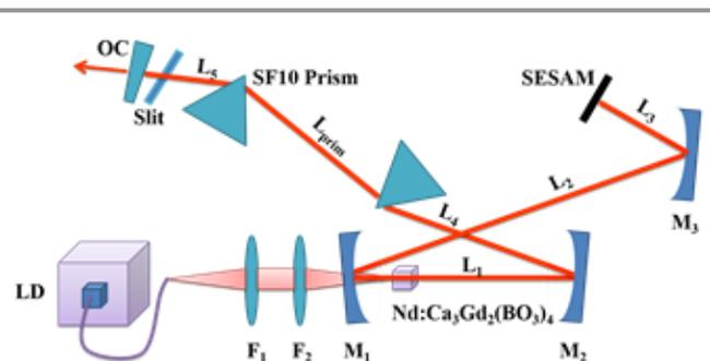
Fig. 1. Schematic of the laser setup. LD, laser diode; F1, F2, lenses with focal length of 100 and 80 mm, respectively; M1, M2 and M3: plano-concave mirrors, ROC—100 mm, -300 mm, and -100 mm, respectively; L1—23.5 cm, L2—59 cm, L3—5 cm, L4—12.5 cm, L5—16 cm, L<sub>prism</sub>—56 cm.
