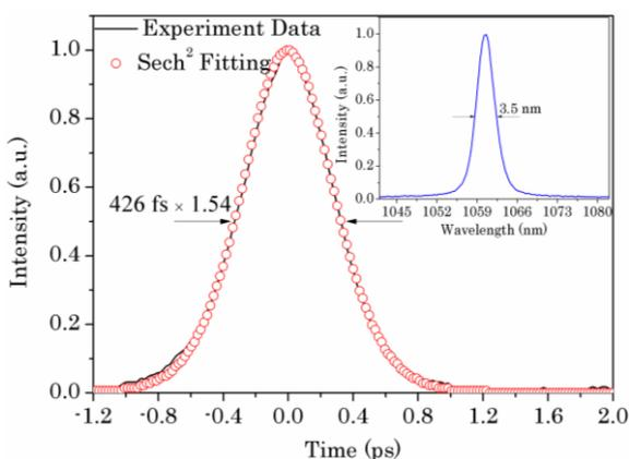
Fig. 8. Autocorrelation trace of mode-locked laser pulses by using 3.5% output coupler. Inset: Spectrum of mode-locked laser with a spectrum FWHM of 3.5 nm at central wavelength of 1061.5 nm
