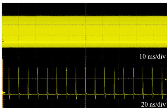
Fig. 4. Mode-locked pulse train recorded on 10 ms and 20 ns per division time scales.
