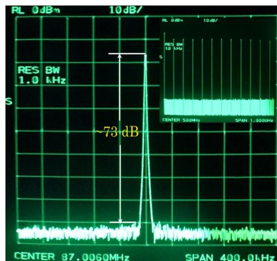
Fig. 5. RF spectrum of the laser output. Insert: RF spectrum up to 1 GHz.
