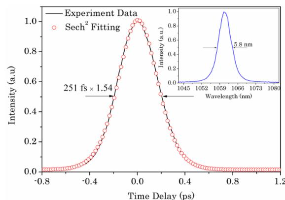
Fig. 6. Autocorrelation trace of mode-locked laser pulses by using 1.6% output coupler. Inset: Spectrum of mode-locked laser pulses with a spectrum FWHM of 5.8 nm at central wavelength of 1061.5 nm.
