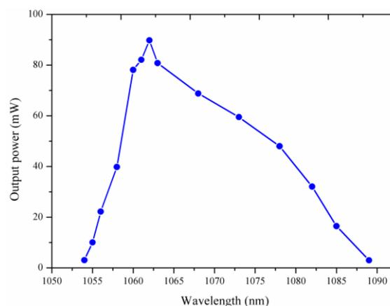
Fig. 2. Wavelength tuning trace of the Nd:Ca<sub>3</sub>Gd<sub>2</sub>(BO<sub>3</sub>)<sub>4</sub> laser.
