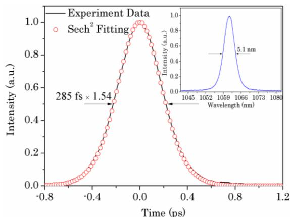
Fig. 7. Autocorrelation trace of mode-locked laser pulses by using 2.4% output coupler. Inset: Spectrum of mode-locked laser with a spectrum FWHM of 5.1 nm at central wavelength of 1061.5 nm
