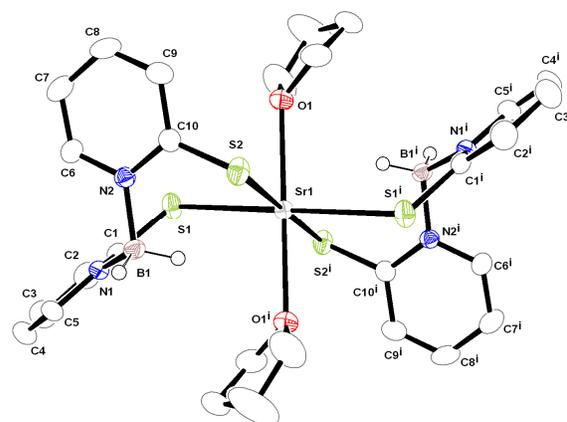
**Figure 2.** Solid-state structure of complex **3** and ellipsoids are drawn to encompass 50% probability. Hydrogen atoms (except H1a, H1b, H1a' and H1b') are omitted for clarity. Selected bond lengths [Å] and bond angles[°]: Sr1–S1 3.0171(8), Sr1–S2 2.991(1), Sr1–O1 2.552(2), Sr1–O1' 2.552(2), Sr1–S1' 3.0171(8), Sr1–S2' 2.991(1). More bond lengths and angles are given in supporting information.
