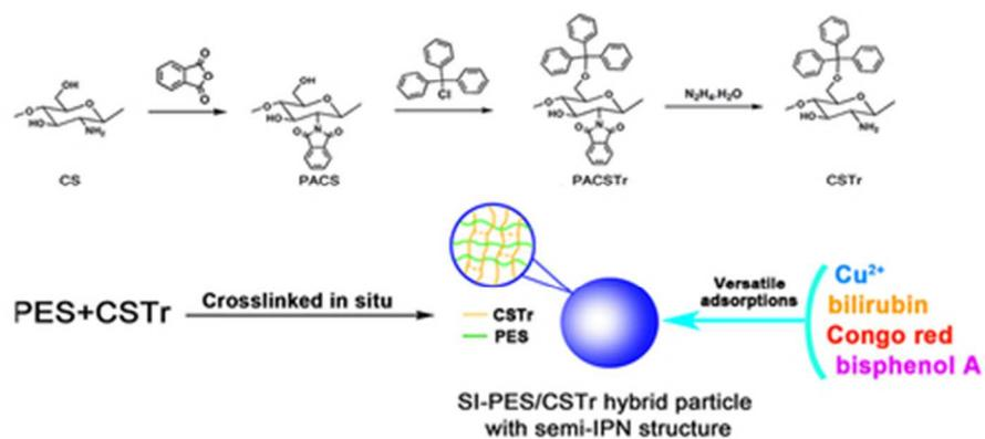
The schematic illustration for preparing PES/CS, PES/CSTr and SI-PES/CSTr particles using Method 1 and Method 2, respectively.
