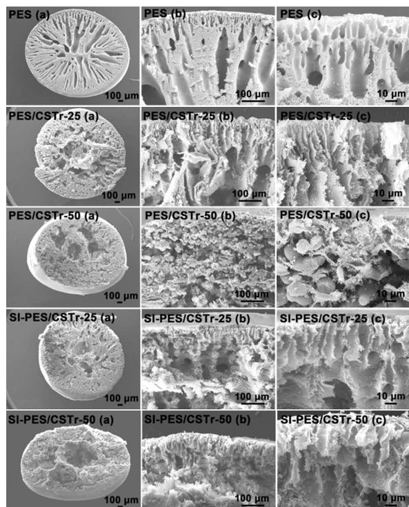
**Figure 3.** SEM pictures of cross-sections for PES, PES/CSTR-25, PES/CSTR-50, SI-PES/CSTR-25 and SI-PES/CSTR-50 particles.
