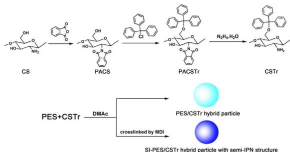
**Scheme 1.** The schematic illustration for preparing PES/CS, PES/CSTr and SI-PES/CSTr particles using Method 1 and Method 2, respectively.
