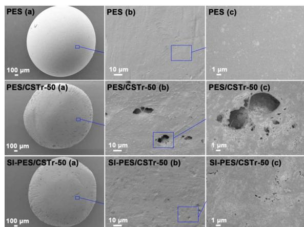
**Figure 4.** SEM pictures of surfaces for PES, PES/CSTR-50, and SI-PES/CSTR-50 particles.
