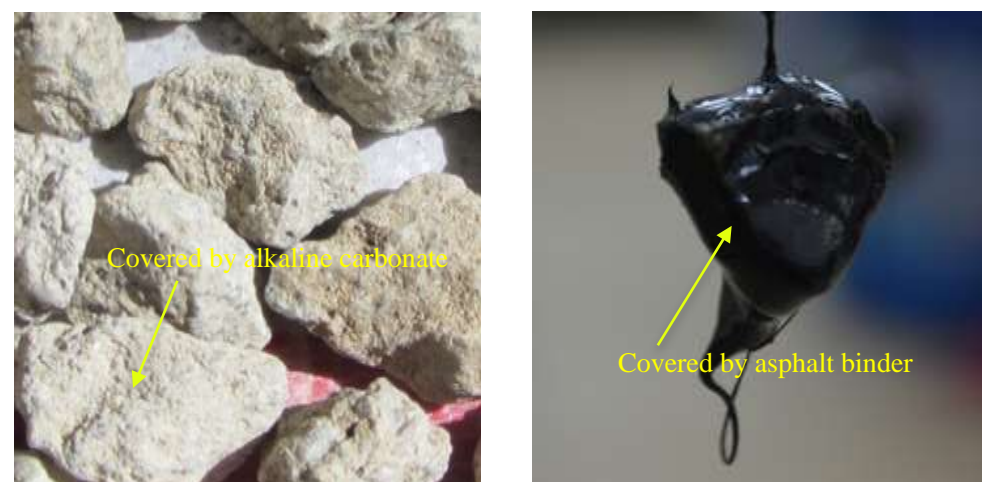
(b) RCA samples covered by alkaline carbonate (left), and full surface covered by asphalt for treated-RCA (right)
