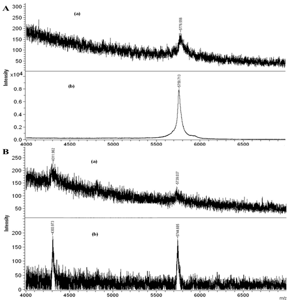
**Figure 3.** MALDI-TOF mass spectra of Insulin (80 nM) using (A) Ag@ODT/AMP and (B) Ag@ODT/TG (a) without AgNPs-SDME, direct analysis of aqueous sample with CHCA (5000 ppm) (b) with AgNPs- SDME and CHCA by using AgNPs- SDME at room temperature for 5 min extraction and stirring at 200 rpm and CHCA (5000 ppm) at pH 4, laser energy 60 %
