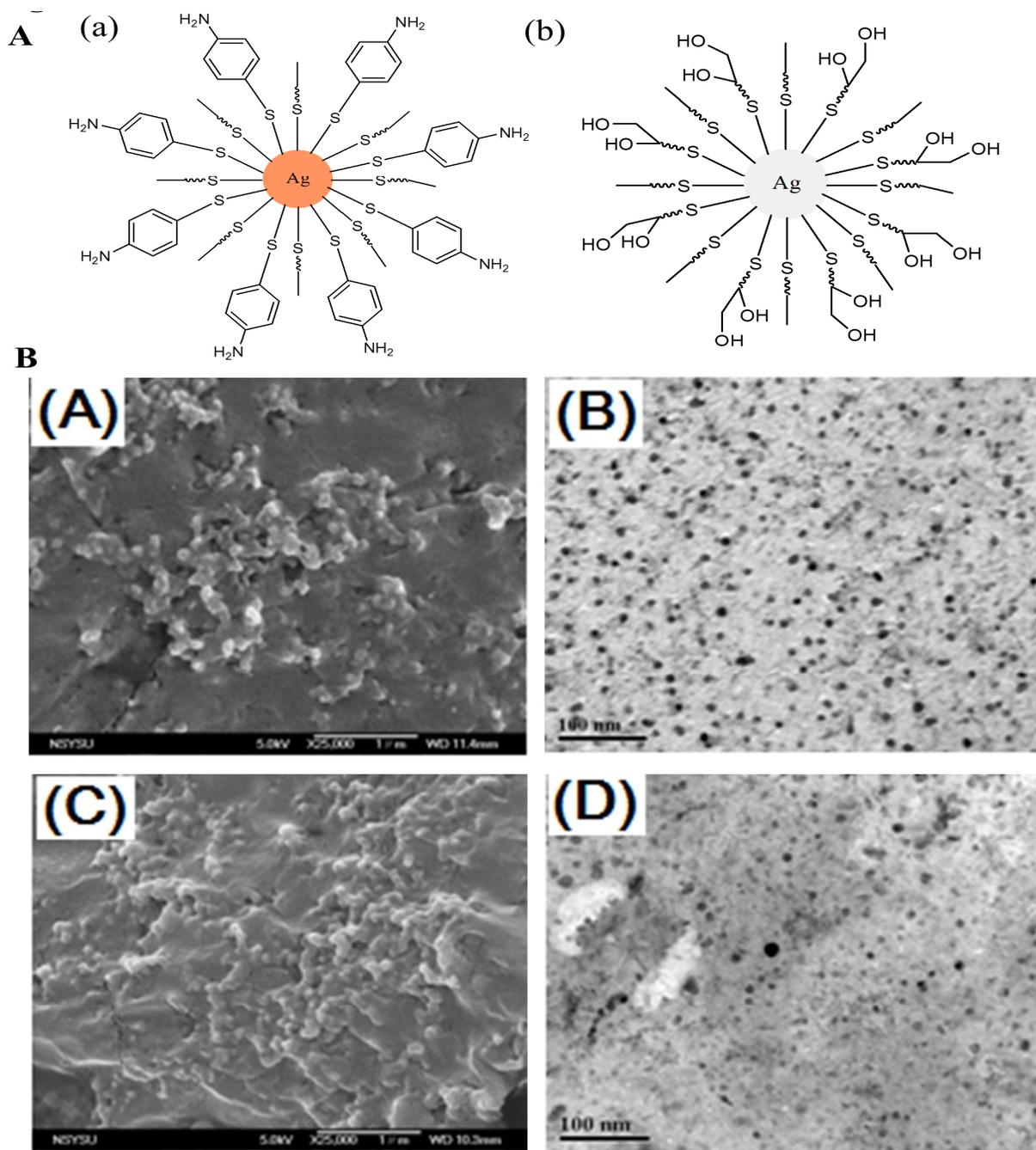
**Figure 1.** (A) Structure of Ag@ODT/AMP and Ag@ODT/TG and (B) their characterization using SEM for (a) Ag@ODT/AMP and (c) Ag@ODT/TG and TEM (b) Ag@ODT/AMP and (d) Ag@ODT/TG
