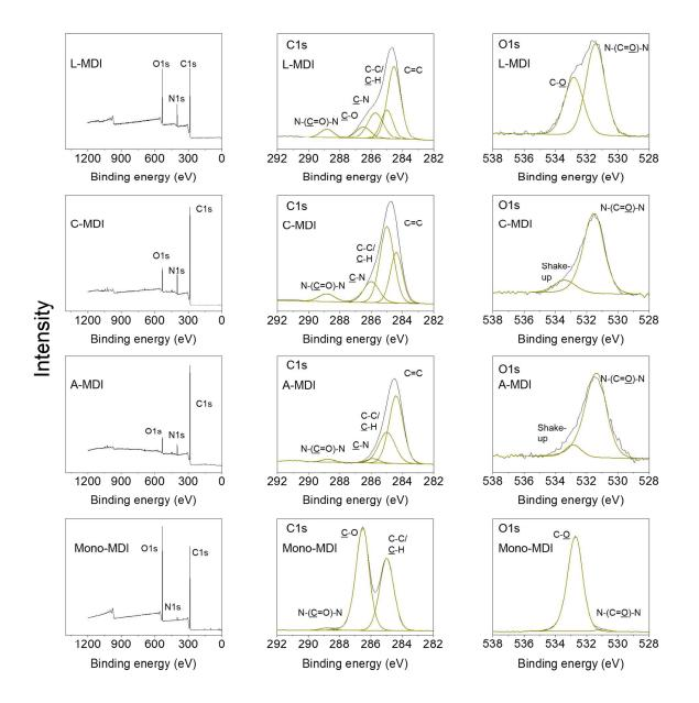
**Figure 5:** *XPS elemental surveys (left) and C 1s (middle) and O 1s (right) spectra of reference compounds L-MDI, C-MDI, A-MDI and Mono-MDI and best fits (see text for more details).*
