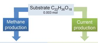
11 mol CO<sub>2</sub> mol<sup>-1</sup> substrate 11 mol CH<sub>4</sub> mol<sup>-1</sup> substrate 22 mol CO<sub>2</sub> mol<sup>-1</sup> substrate 88 mol H<sup>+</sup> mol<sup>-1</sup> substrate 88 mol electrons mol<sup>-1</sup> substrate
