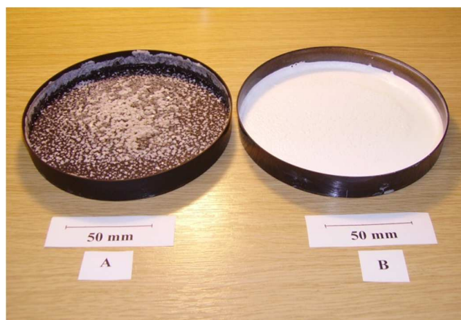
Figure 3. Unfoamed evaporated sea-salt solution (35 gL -1 ) (A) without additives and (B) with 0.5 wt.% HPMC (Methocel™ E50). The dishes were polystyrene Petri dishes of 135 mm diameter sprayed with matt black paint. They were filled to a height of 15 mm giving 0.53 kg m -2 salt residue. The reflectance measurements are given in Table 2.
