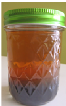
Figure 2. Small scale biodiesel reaction at Maine Standard Biofuels (MSB). Biodiesel/methyl esters (top), soaps (middle), crude glycerin (bottom).
