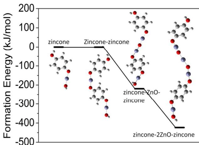
**Fig. 6** Formation energies of a single zincone, double zincone, zincone-ZnO-zincone and zincone-2ZnO-zincone molecular chain as calculated from DFT considering single zincone molecule as the unit building block.
