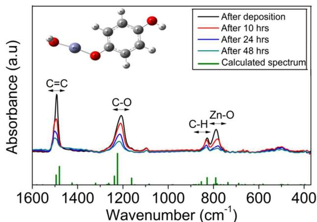
**Fig. 2** FTIR spectra of 300 cycles of zincone film grown on KBr pallets and recorded over a time span of 48 hours. The sample under observation was exposed to ambient condition of 25°C temperature and 60-70% humidity between each scan; Spectrum of 2 MLD zincone cycles obtained from DFT calculations.
