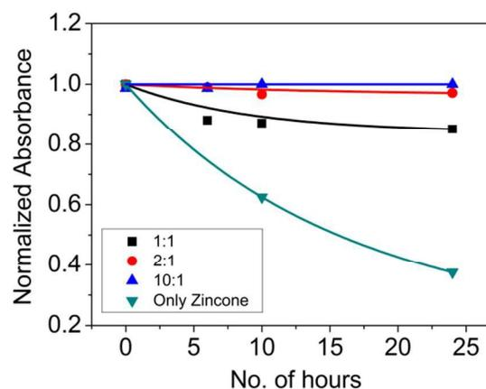
Fig. 5 Variation in the absorbance intensity of Zn-O stretch at  $788\text{cm}^{-1}$  position with time with inclusion of 0,1,2 and 10 Zn-O moieties between each zincone molecule.
