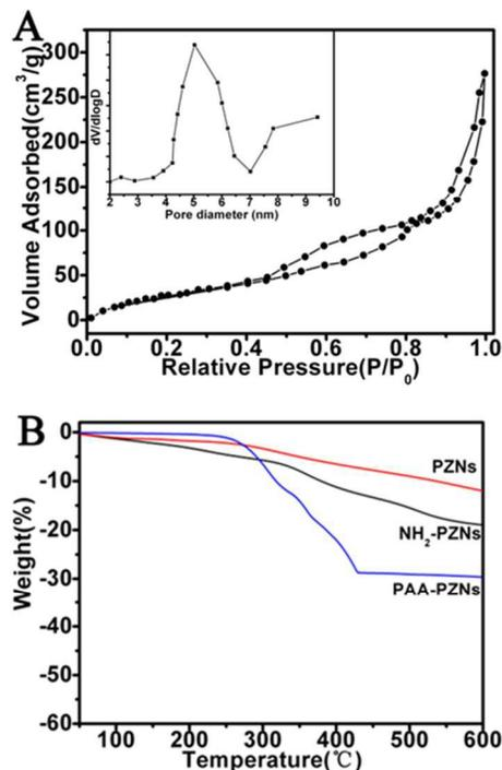
Figure 3 (A) Nitrogen adsorption–desorption isotherms and pore size distribution plot (inset) of PZNs. (B) TGA curves of PZNs, NH<sub>2</sub>-PZNs, and PAA-PZNs.
