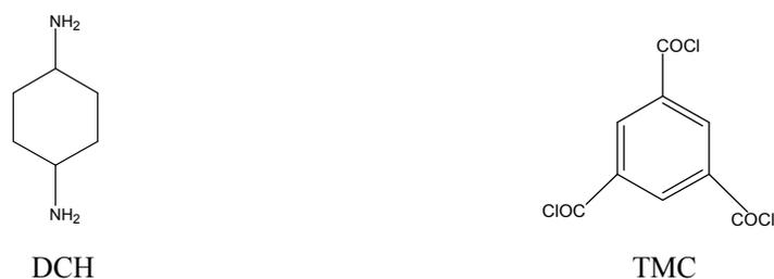
**Fig.1. Chemical structure of the monomers used: 1,4-Diaminocyclohexane (DCH) and trimesoyl chloride (TMC).**
