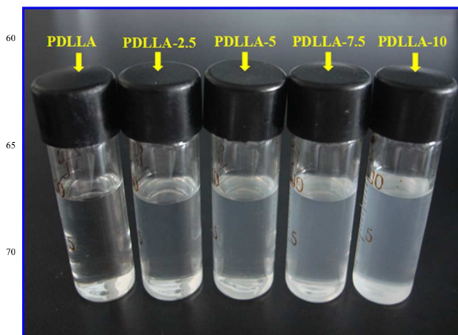
Fig.6. The photos of the solutions of the prepared samples for neat PDLLA, PDLLA2.5, PDLLA5, PDLLA7.5, and PDLLA10, after dissolving in acetone without stirring.
