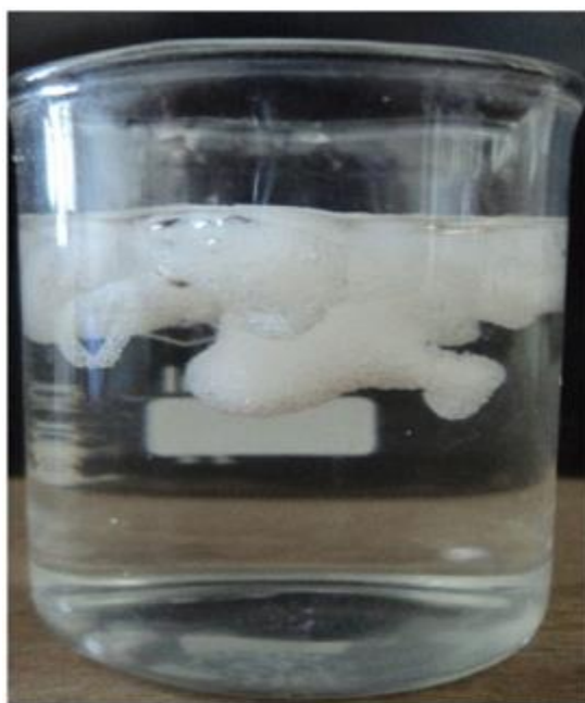
Fig. 2 Photograph showing the formation of gellan gel in simulated gastric fluid pH 1.2.
