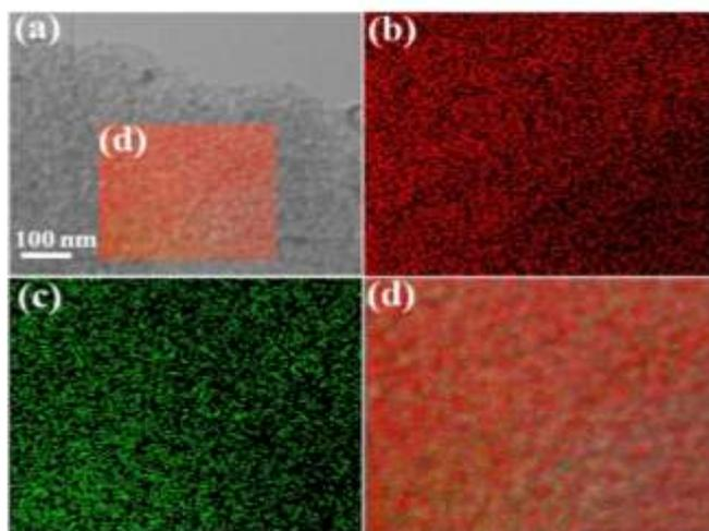
**Fig. 6** (a) Selected area of SCAC-60 composite subjected to elemental mapping (b) carbon (c) sulfur and (d) cumulative carbon elemental mapping image.
