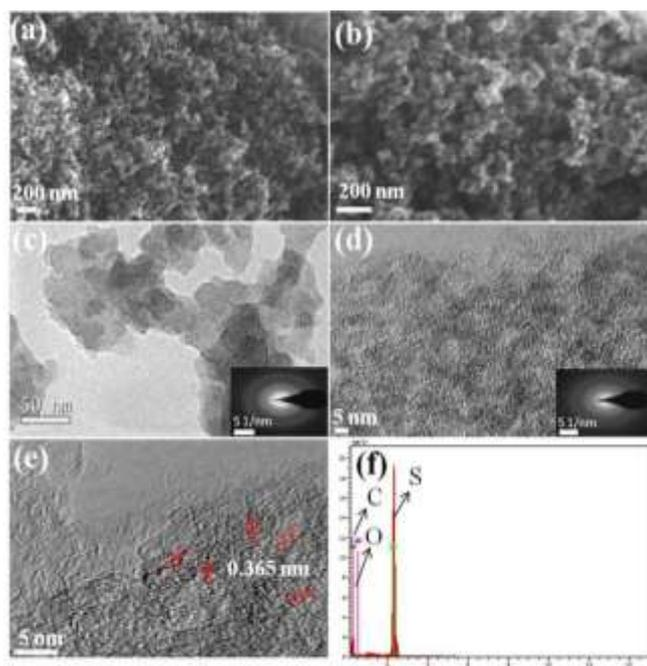
**Fig. 5** (a) Low and (b) high magnification FESEM images of carbon aerogel (c) TEM image (inset-SEAD pattern) of carbon aerogel (d) Low and (e) high magnification HRTEM images (inset-SEAD pattern) and (f) EDX spectrum of 60 wt. % of sulfur loaded carbon aerogel.
