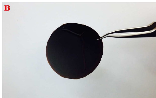
Figure 1: A) Schematic representation showing the synthetic procedure for the formation of nisin antimicrobials peptide attached 3D graphene oxide. B) Photograph shows the foam membrane formed from graphene oxide membrane with antimicrobial nisin peptides attached.
