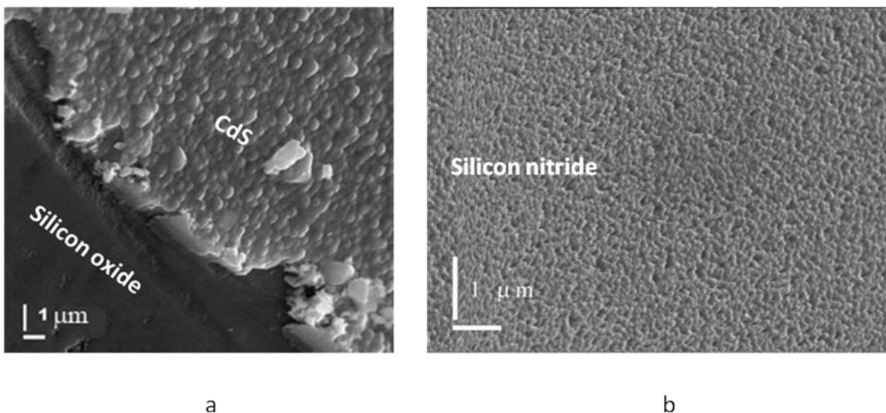
**Figure 3.** SEM images of (a) silicon oxide and (b) silicon nitride surfaces after the CdS deposition process performed under the same conditions. CdS layer is seen only in (a) and its edge is shown for clarity.
