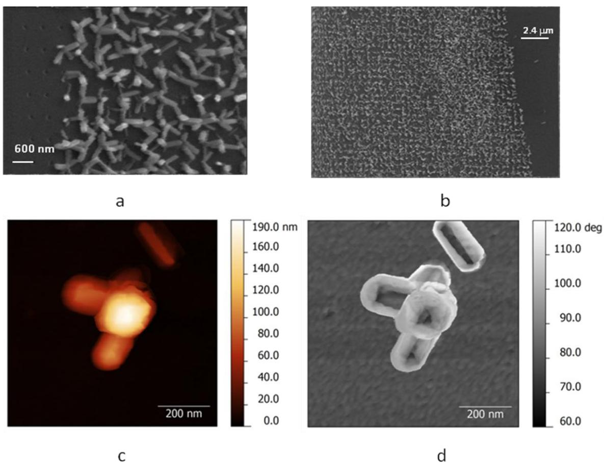
**Figure 1.** (a,b) SEM images of tetrapod nanocrystal arrays grown in cavities of the silicon nitride surface; the cavities regularly cover the whole  $\text{Si}_3\text{N}_4$  surface, however, some holes in (a) survived the deposition procedure due to incomplete etching. AFM of (c) topography and (d) phase image of a single tetrapod CdS crystal; one arm has been broken.
