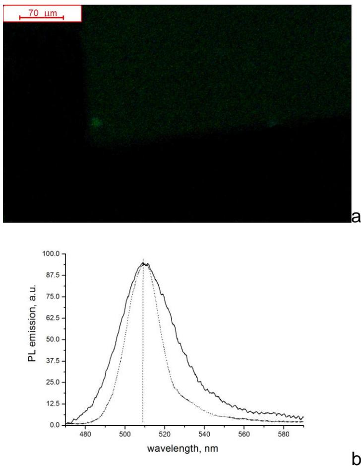
**Figure 2.** (a) Fluorescence microscopy image (the shape of the emitted region conforms that of a separate cavity array of the patterned substrate (Fig.S1)) and (b) PL emission spectrum of the array of CdS tetrapod nanocrystals (solid curve) compared with PL emission of the single CdS crystal (dotted curve, adapted from ref. [27]).
