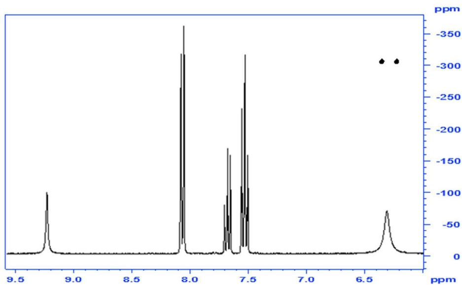
**Figure 1:**  $^1\text{H}\times^{15}\text{N}$  NMR correlation spectrum of compound **2**, the *N*-benzoylated product of HU; inset:  $^1\text{H}$ - $^1\text{D}$  spectrum
