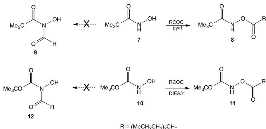
**Scheme 3:** *O*-Acylation of a hydroxamic acid and an *N*-hydroxycarbamate
