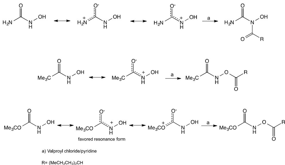
**Scheme 4:** Some suggested resonance structures and the obtained acylation products of HU, a hydroxamic acid and an *N*-hydroxycarbamate
